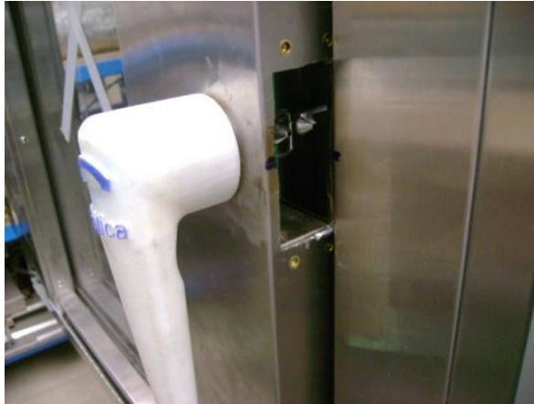
Fig. 9. New lock assembled for a test
