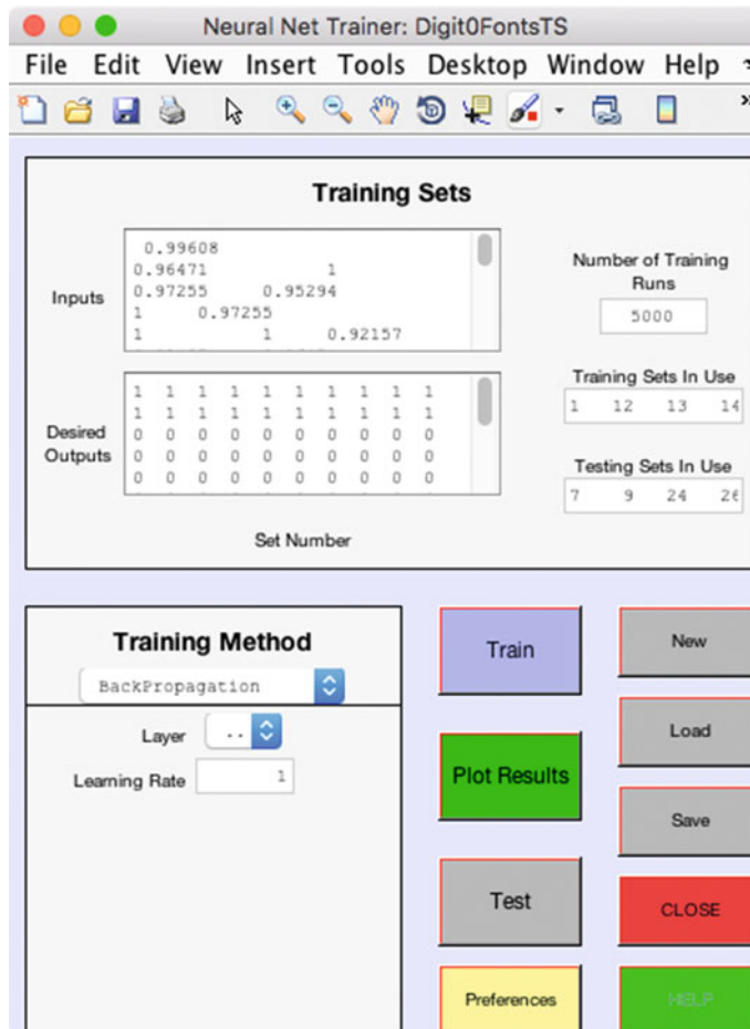
Figure 9.5: The neural net training GUI opens when the train button is clicked in the developer.
