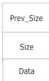
Figure 32.0 Heap Memory from dlmalloc 's view.
