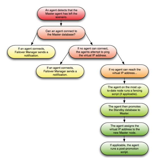
Fig. 3: Confirming the failure of the Master Agent.
