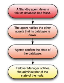
Fig. 2: Confirming the failure of a Standby Database.
