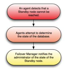
Fig. 4: Failure of Standby Agent.
