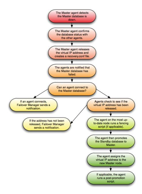
Fig. 1: Confirming the Failure of the Master Database.
