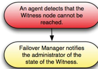
Fig. 5: *Confirming the Failure of a dedicated Witness.*
