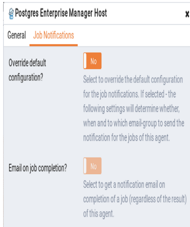
Fig. 4.14: Job notification configuration: agent level
