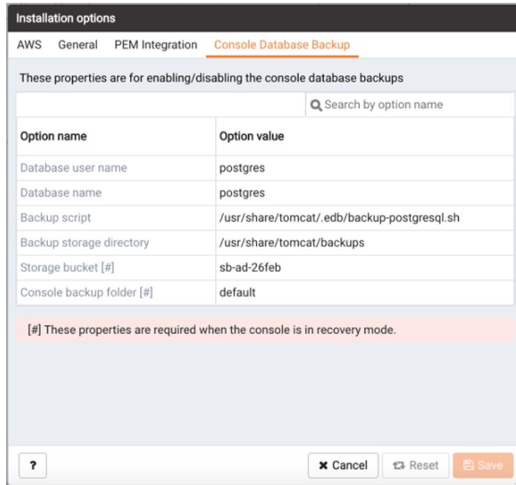
Fig. 8: The Console database backup tab
