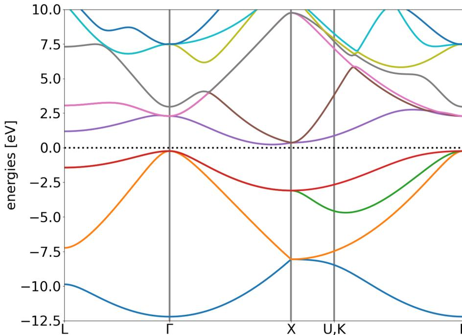
Figure 2: Bandstructure of silicon as calculated with GPAW. Energies are given relative to the Fermi energy. Although the band gap is too narrow, all important features have been reproduced qualitatively correct.
