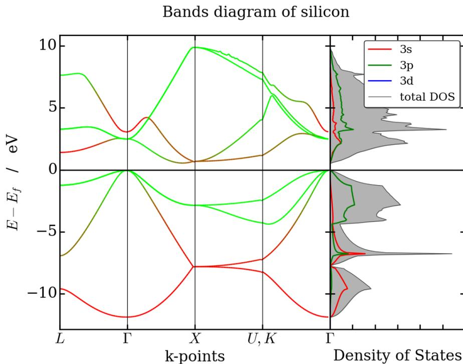
Figure 3: Bandstructure of silicon colored according to projected density of states on 3s and 3p atom orbitals. Provided by G.S. Vallverdu under MIT license: [https://github.com/gVallverdu/bandstructureplots/blob/master/Si\\_bands/bands\\_Si.png](https://github.com/gVallverdu/bandstructureplots/blob/master/Si_bands/bands_Si.png).
