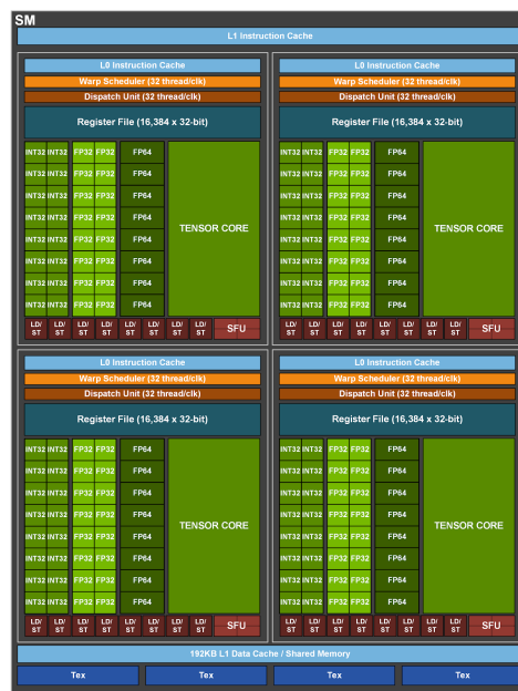
Figure 6.5: Simplified block diagram of an NVIDIA Ampere Streaming Multiprocessor (SM).
