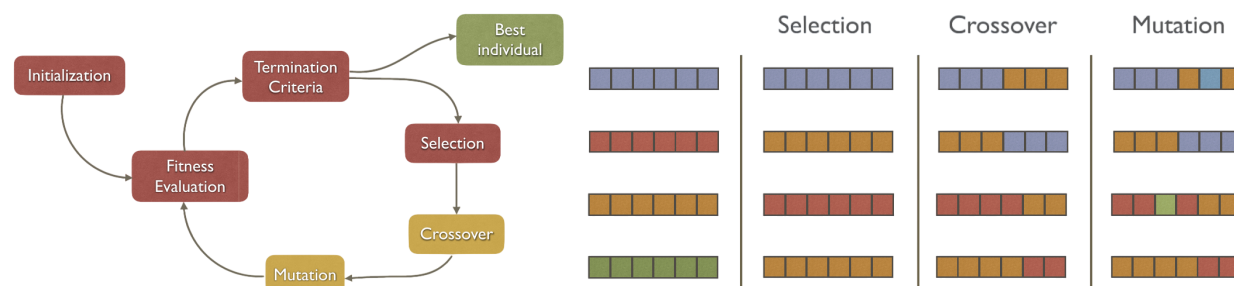
Figure 2.1: Left: Diagram showing the main components and their interactions in the evolutionary process. Right: Example of genetic operators (selection, crossover, mutation) acting on binary strings.
