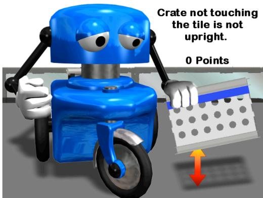
This picture shows a robot still holding a crate at the end of the autonomous period. This crate will not score because the crate does not have at least one bottom edge of the crate touching the field.
