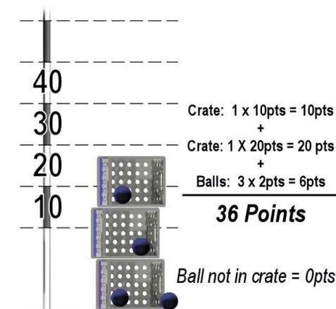
This example is similar to the one above however there is a ball scored in each crate in the stack. The balls are completely supported by the crate and nothing else except the one that is just resting on the field mat. So 3 balls are scored (6 points) and 3 crates are stacked – 1 in the 0 point range (the bottom one), 1 in the 10 point range, and 1 in the 20 point range. *Stacking bonus* is 30 points; ball scoring is 6 points for a total of 36 points.
