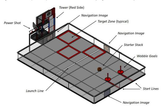
Figure 4.3-1 – Isometric view of the *Playing Field (red)*
