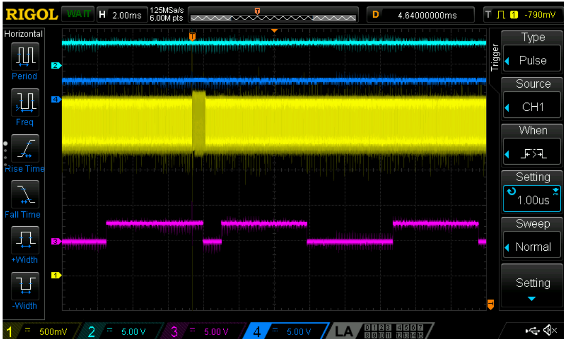
Figure 13: The CC2541 pin toggling application with a 90ns crowbar glitch at trigger T , causing a reset, visible in the pattern in trace 1 and the initial 1ms pin toggle in trace 3, at the start of the application. Trace 1 (yellow): DCOUPL, trace 2 (light blue): RESET_N, trace 3 (purple): STATE on the development board (the pin being toggled), trace 4 (dark blue): Debug Data.
