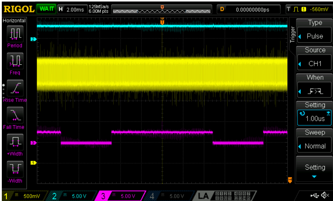
Figure 12: The CC2541 pin toggling application with a 50ns crowbar glitch at trigger T , causing the pin toggle instruction to be skipped and the STATE pin remains high for another 5ms. Trace 1 (yellow): DCOUPL, trace 2 (light blue): RESET_N, trace 3 (purple): STATE on the development board (the pin being toggled).
