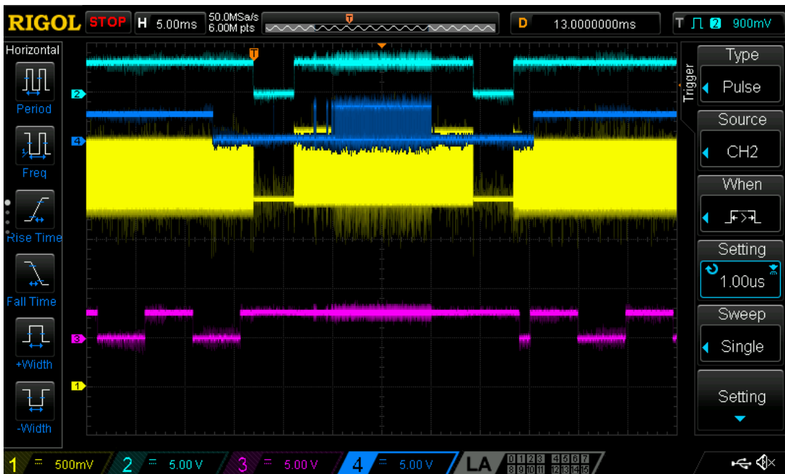
Figure 14: Using cc-tool to read basic info about the CC2541: what its debug status is and its name and flags. Trace 1 (yellow): DCOUPL, trace 2 (light blue): RESET_N, trace 3 (purple): STATE on the development board (the pin being toggled), trace 4 (dark blue): Debug Data.
