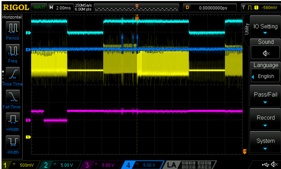
Figure 15: The CC2541 glitch during debug communication which was initially thought to be successful. Notice how trace 3 doesn’t start toggling again because the application has been wiped. Trace 1 (yellow): DCOUPL, trace 2 (light blue): RESET_N, trace 3 (purple): STATE on the development board (the pin being toggled), trace 4 (dark blue): Debug Data.
