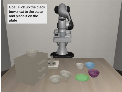
((a)) VLA Pruning Visualization. Grey objects in the scene have been pruned away, while objects with colored mask overlays are identified as semantically and spatially goal relevant. The goal (masked green) and target objects (masked purple) are selected. In addition, a second distractor goal is selected due to ambiguity in the prompt.
