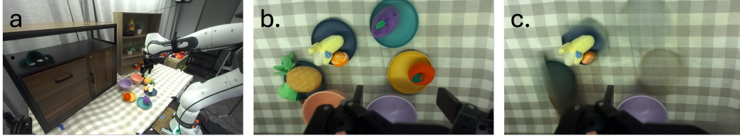
Figure 8: Real hardware VLA experiment. LENS is applied directly on hand image (b) without simulator bounding boxes. Foundation models [32–34] are used to segment and inpaint scenes (c). Performance improvements persist, supporting the validity of the simulation comparison.
