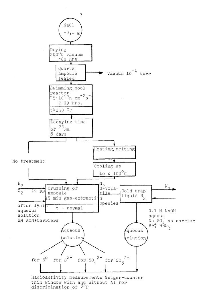
Fig. 1 Scheme of experimental work
