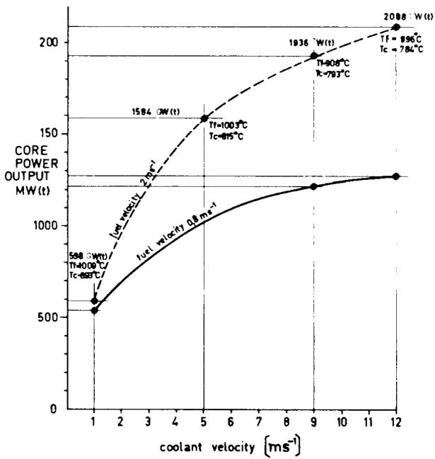
Fig. 8.18 Core power output versus fuel velocity
