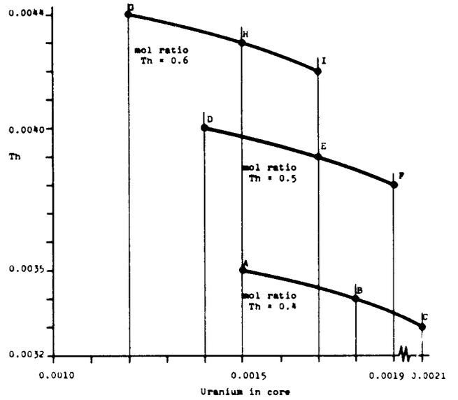
Fig. 3.3 Uranium concentrations for given geometry (THOCL-301) for A, B, C, D, E, F, G, H, I.
