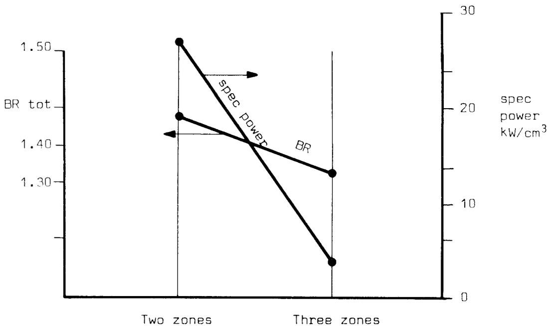
Table 3.17 Three zones reactor: fluoride uranium-plutonium fuel
