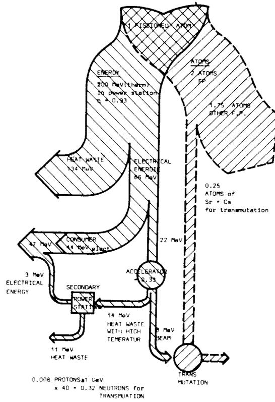
Fig. 4.4 Neutron balance
