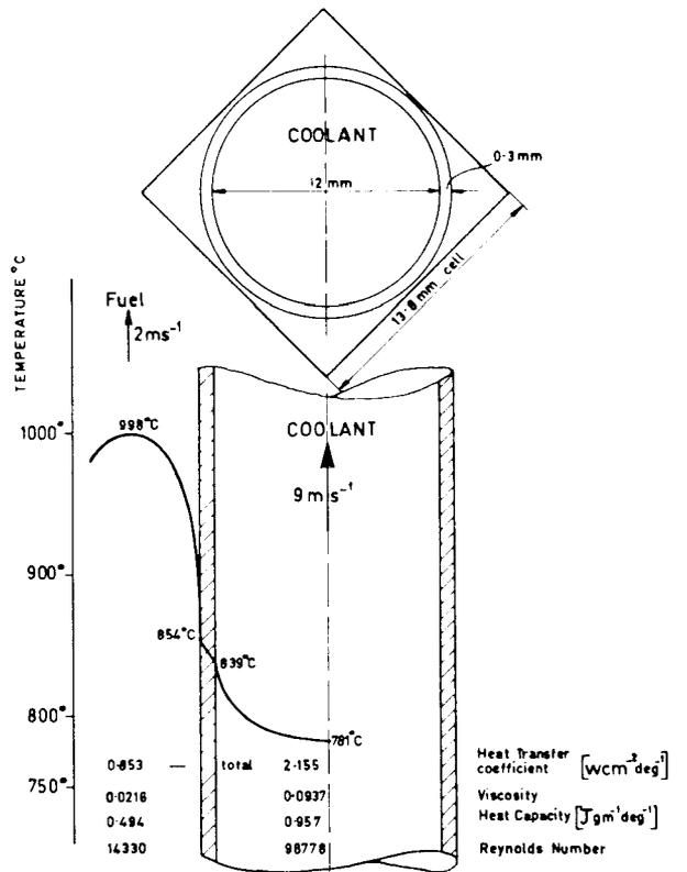
For other pitches between 1.2 and 2.2 and for two selected fuel and sodium velocities values can be seen in Fig. 8.11. The reference case was arbitrarily chosen (see Fig. 8.11). The geometry of the heat exchanger for this reference case is shown in Fig. 8.12. Further parameters are summarised in table 8.4.
