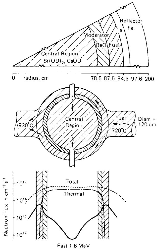
Table 4.6 Geometry and Neutronics of the High-Flux Burner Reactor
