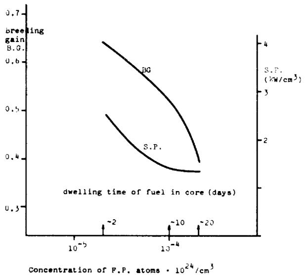
In the steady state reactor a concentration of  $2 \times 10^{-5}$  atoms F.P.  $\times 10^{24}/\text{cm}^3$  for a fuel having  $2.1 \times 10^{-3}$  atoms  $P \times 10^{24}/\text{cm}^3$  is reached for a specific power of  $2 \text{ GW}/\text{m}^3$  after a time  $t$  of
