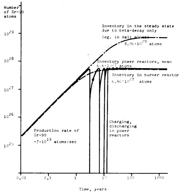
Fig. 4.22 Variant of the beta fission products: Sr-90 and Cs-137
