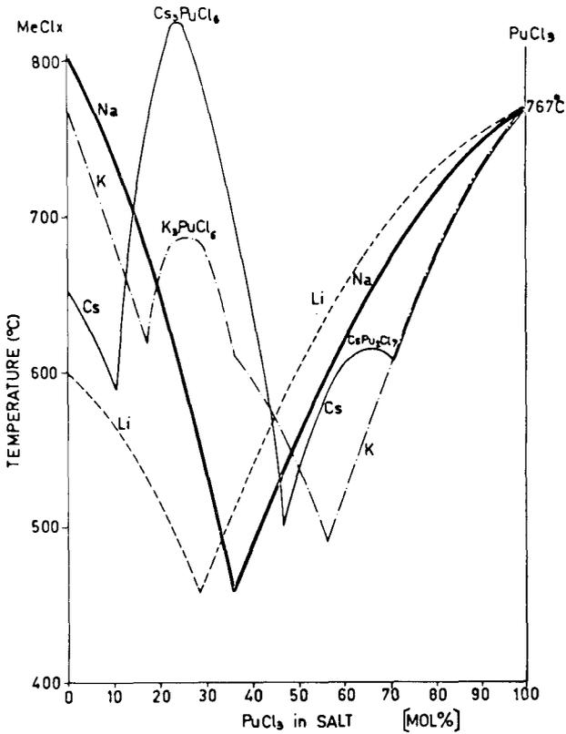
Fig. 6.8 Phase Diagram for PuCl<sub>3</sub>/NaCl and UCl<sub>3</sub>/NaCl
