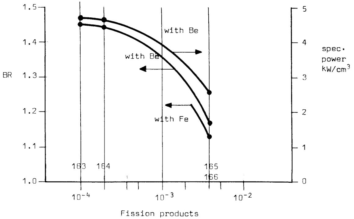
Fig. 3.17 Impact of the beryllium and iron moderator on BR and spec. power
