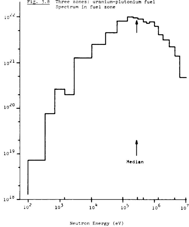
Table 3.7 Three Zone reactor: uranium-plutonium fuel
