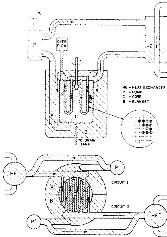
Table 5.2 Molten chloride fast breeder reactor (MCFBR)
