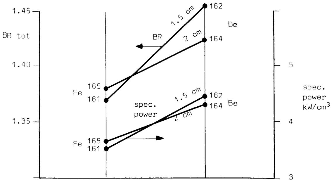
Table 3.15a Three zone reactor: fluoride uranium-plutonium fuel
