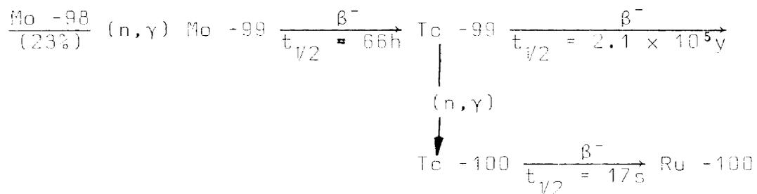
For approx 1000 kg molybdenum in the core in the form of cooling tubes or about 10,000 moles, the Mo-98 gives 2300 mol. The irradiation rate  $N$  (mols/s) equals
