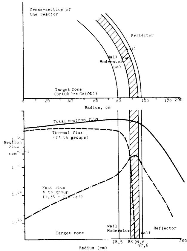
Considering chemical and physical properties, the logical materials to be used inside the flux trap are hydroxide and/or deuterium oxide compounds of the FP. Fig. 4.14A shows that just a small proportion of H molar fraction has a large deleterious effect on the Cs-137 transmutation rate. This is due to the H absorption cross section. Therefore, CsOD and Sr(OD)<sub>2</sub> are preferred.
