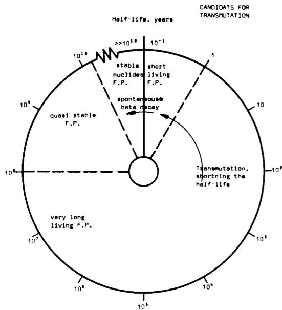
Table 4.2 Possibility for transmutation of F.P. - particularly Cs-137 and Sr-90 in a fission reactor according to BNWL - 1900
