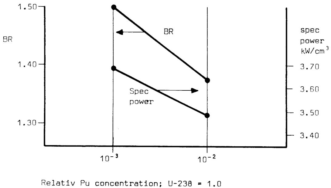
Table 3.16a Three zones reactor: fluoride uranium-plutonium fuel
