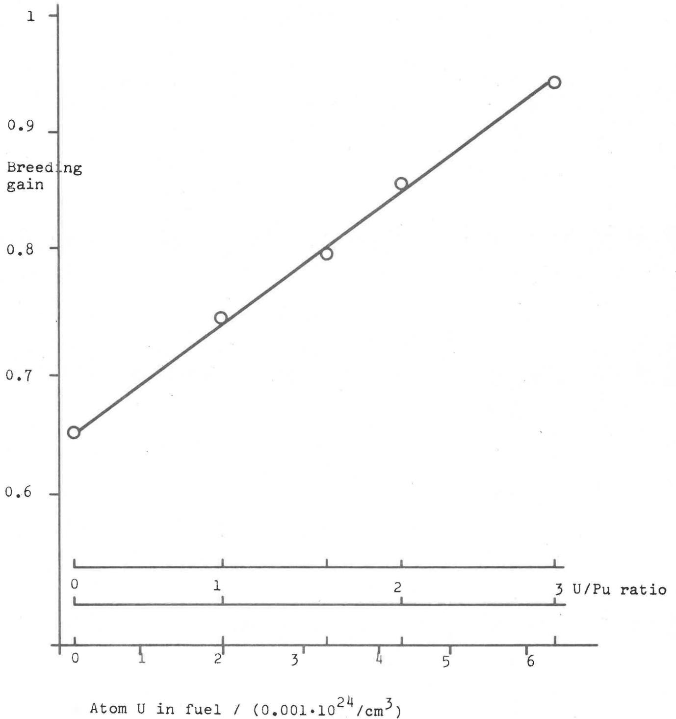
Fig. 8 Impact of Uranium Concentration in the Fuel
