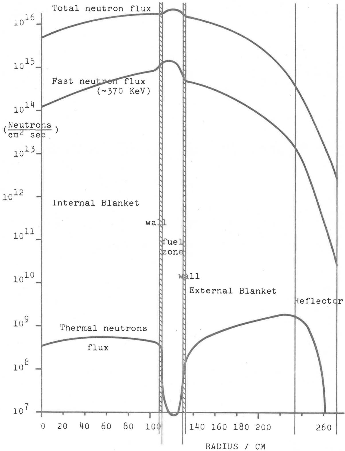
Fig. 3' Total Flux in the Fuel Zone
