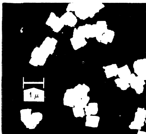
(a) Cubic Shape From 10°C Precipitated Oxalate
