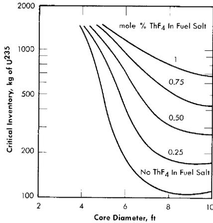
FIG. 14-3. Initial critical inventories of  $U^{235}$  in two-region, homogeneous, molten fluoride-salt reactors. External fuel volume,  $339 \text{ ft}^3$ .
