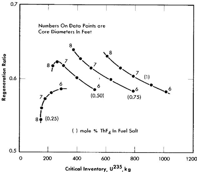
FIG. 14-7. Initial fuel regeneration in two-region, homogeneous, molten fluoride-salt reactors fueled with  $U^{235}$ . Total power, 600 Mw (heat); external fuel volume, 339 ft<sup>3</sup>; core and blanket salts No. 2.
