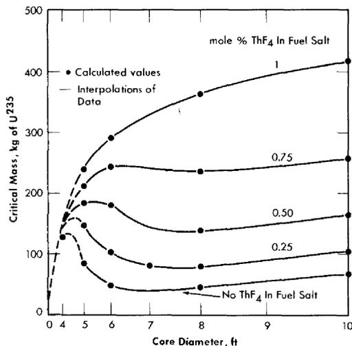
FIG. 14-2. Initial critical masses of  $U^{235}$  in two-region, homogeneous, molten fluoride-salt reactors.
