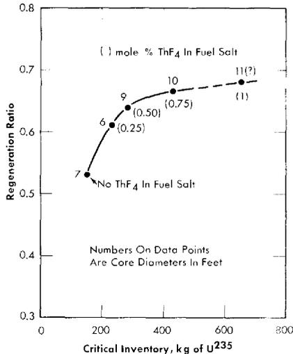
FIG. 14-5. Maximum initial regeneration ratios in two-region, homogeneous, molten fluoride-salt reactors fueled with  $U^{235}$ . Total power, 600 Mw (heat); external fuel volume, 339 ft<sup>3</sup>.
