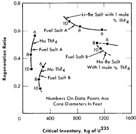
FIG. 14-8. Comparison of regeneration ratio and critical inventory in two-region, homogeneous, molten fluoride-salt reactors fueled with  $U^{235}$ . Fuel salt A: 37 mole %  $BeF_2$  plus 63 mole %  $LiF$ . Fuel salt B: 46 mole %  $BeF_2$  plus 54 mole %  $NaF$ .
