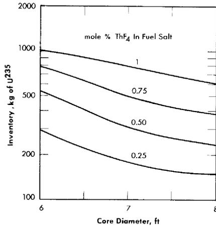
FIG. 14-6. Initial critical inventories of  $U^{235}$  in two-region, homogeneous, molten fluoride-salt reactors. Total power, 600 Mw (heat); external fuel volume, 339 ft<sup>3</sup>; core and blanket salts No. 2.
