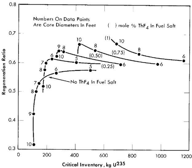
FIG. 14-4. Initial fuel regeneration in two-region, homogeneous, molten fluoride-salt reactors fueled with  $U^{235}$ . Total power, 600 Mw (heat); external fuel volume,  $339 \text{ ft}^3$ ; core and blanket salts No. 1.
