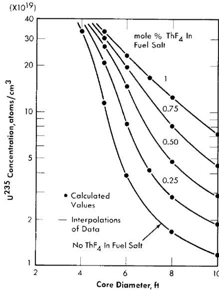
FIG. 14-1. Initial critical concentration of  $U^{235}$  in two-region, homogeneous, molten fluoride-salt reactors.
