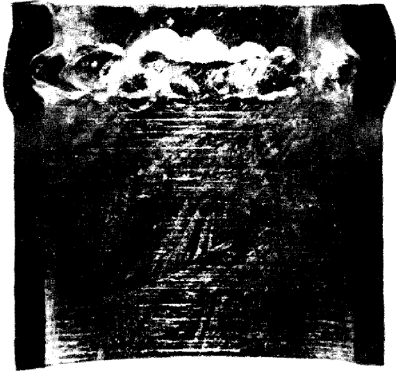
FIG. 21-8. Preferential attack on 5% Cr- \frac{1}{2} % Mo Weld in HVL I-Run 4.
