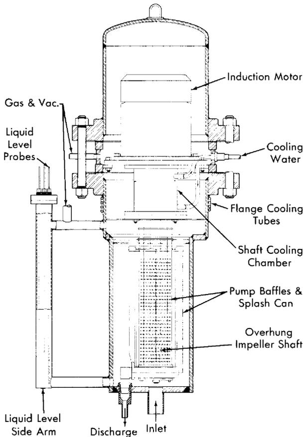
FIG. 23-5. Canned-motor centrifugal pump developed at Brookhaven.
