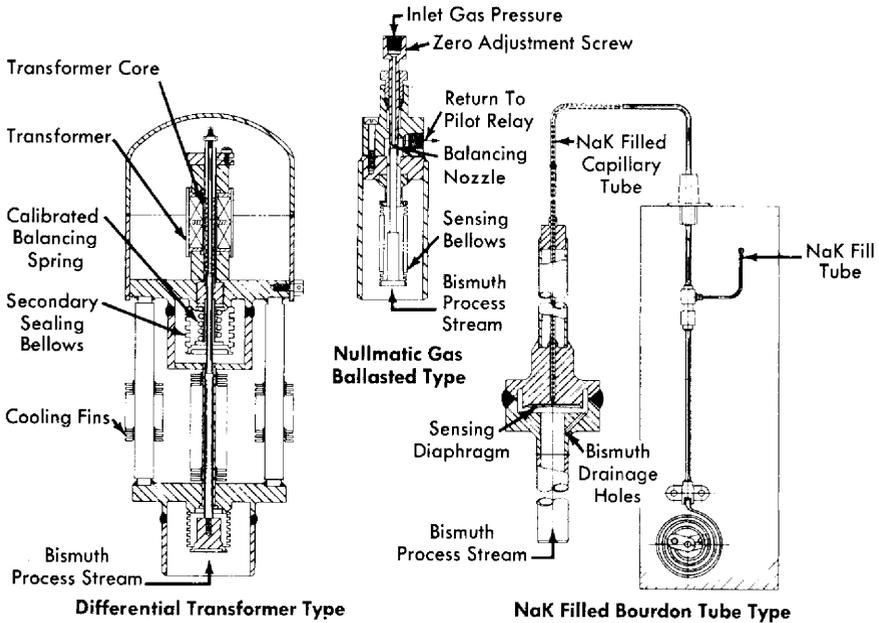
FIG. 23-9. Pressure transmitters.
