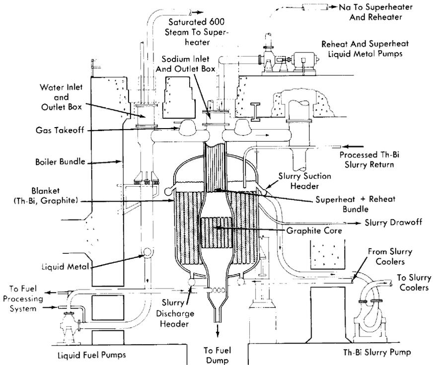
FIG. 23-2. Externally cooled open-cycle arrangement LMFR.
