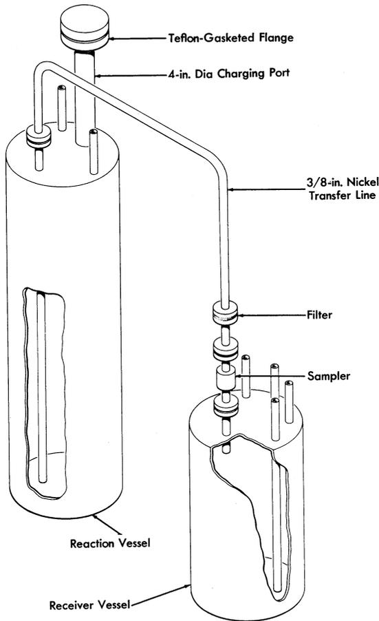
FIG. 12-11. Diagram of purification and storage system.
