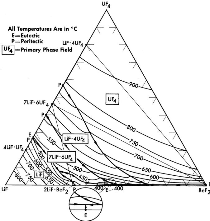
FIG. 12-7. The system LiF-BeF<sub>2</sub>-UF<sub>4</sub>.
