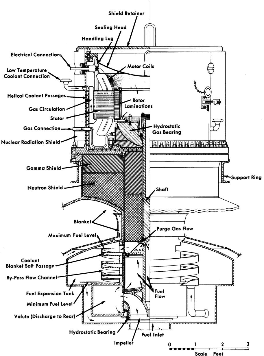
FIG. 15-3. Improved molten-salt fuel pump designed for power reactor use. Operating temperature,  $1200^{\circ}\text{F}$ ; flow rate, 24,000 gpm; head, 70 ft of fluid.
