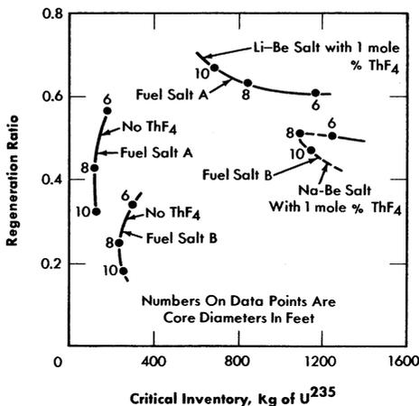
FIG. 14-8. Comparison of regeneration ratio and critical inventory in two-region, homogeneous, molten fluoride-salt reactors fueled with U<sup>235</sup>. Fuel salt A: 37 mole % BeF<sub>2</sub> plus 63 mole % Li<sup>7</sup>F. Fuel salt B: 46 mole % BeF<sub>2</sub> plus 54 mole % NaF.
