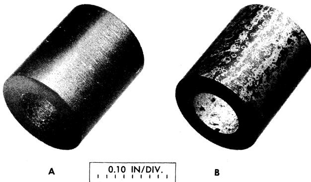
FIG. 13-23. CCN graphite (A) before and (B) after exposure for 1000 hr to  $\text{NaF-ZrF}_4\text{-UF}_4$  (50-46-4 mole %) at 1300°F as an insert in the hot leg of a thermal-convection loop. Nominal bulk density of graphite specimen: 1.9 g/cm<sup>3</sup>.
