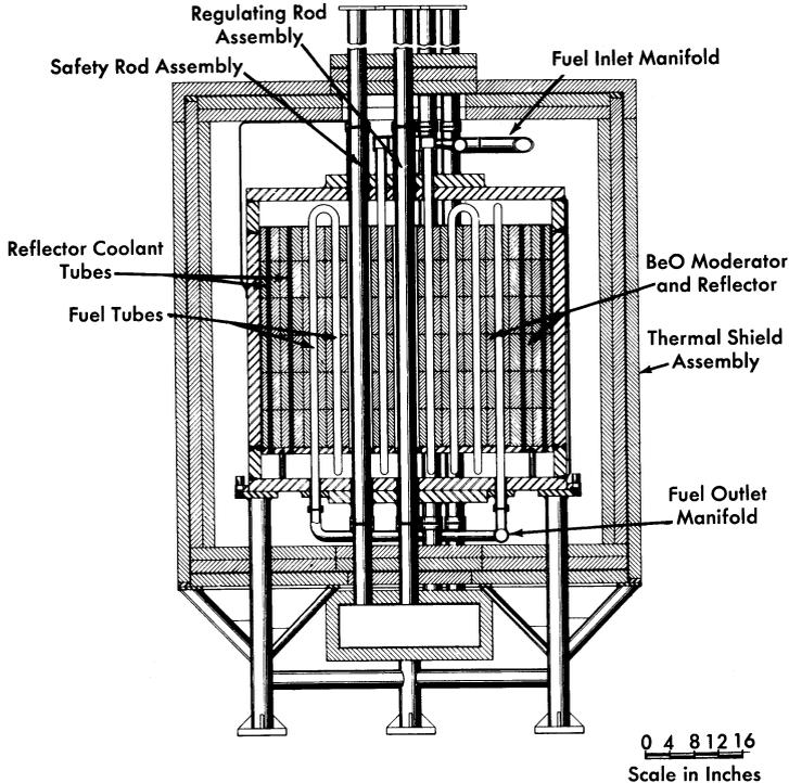
FIG. 16-2. Elevative section of the Aircraft Reactor Experiment.
