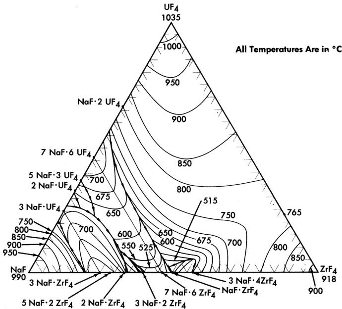
FIG. 12-6. The system NaF-ZrF<sub>4</sub>-UF<sub>4</sub>.
