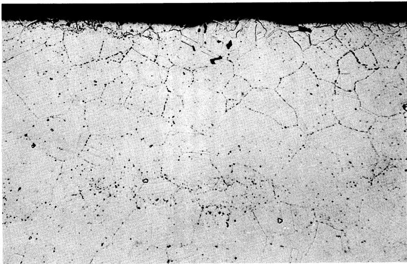
FIG. 13-4. Hot-leg section of Inconel thermal-convection loop which circulated the fuel mixture NaF-ZrF<sub>4</sub>-UF<sub>4</sub> (55.3-40.7-4 mole %) for 1000 hr at 1250°F. (250×)
