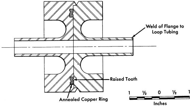
FIG. 15-7. Indented-seal flange.
