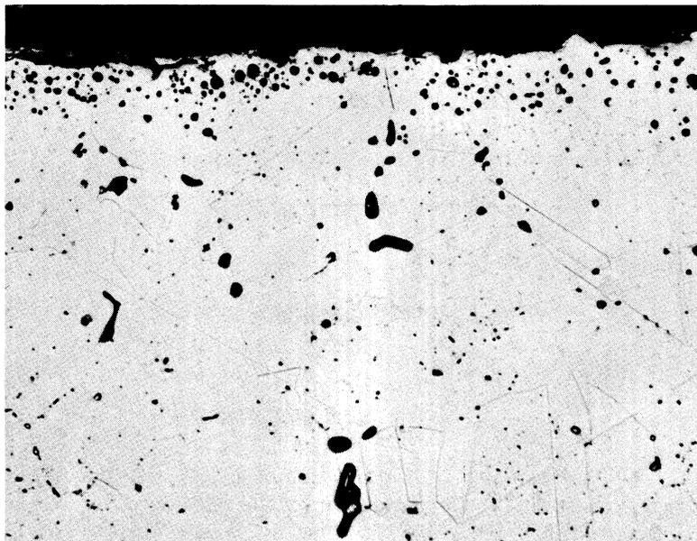
FIG. 13-3. Hot-leg section from an Inconel thermal-convection loop which circulated the fuel mixture  $\text{NaF-ZrF}_4\text{-UF}_4$  (50-46-4 mole %) for 1000 hr at  $1500^\circ\text{F}$ . (250 $\times$ )
