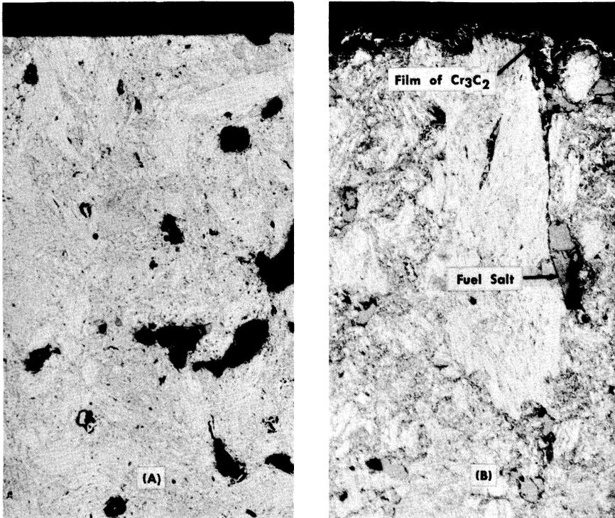
FIG. 13-24. Cross sections of samples shown in Fig. 13-23. (A) Before exposure; (B) after exposure. Note the thin film of  $\text{Cr}_3\text{C}_2$  on the surface in (B). The black areas in (A) are pores. In (B) the pores are filled with salt. (100 $\times$ )
