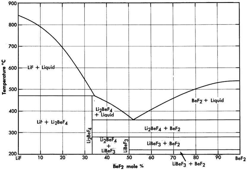
FIG. 12-3. The system LiF-BeF<sub>2</sub>.
