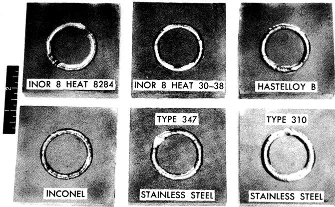
FIG. 13-7. Circular-groove tests of weld metal cracking.
