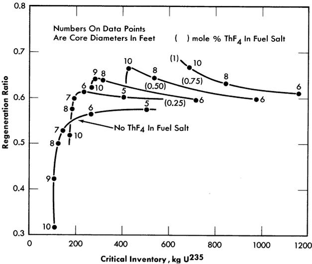
FIG. 14-4. Initial fuel regeneration in two-region, homogeneous, molten fluoride-salt reactors fueled with U<sup>235</sup>. Total power, 600 Mw (heat); external fuel volume, 339 ft<sup>3</sup>; core and blanket salts No. 1.
