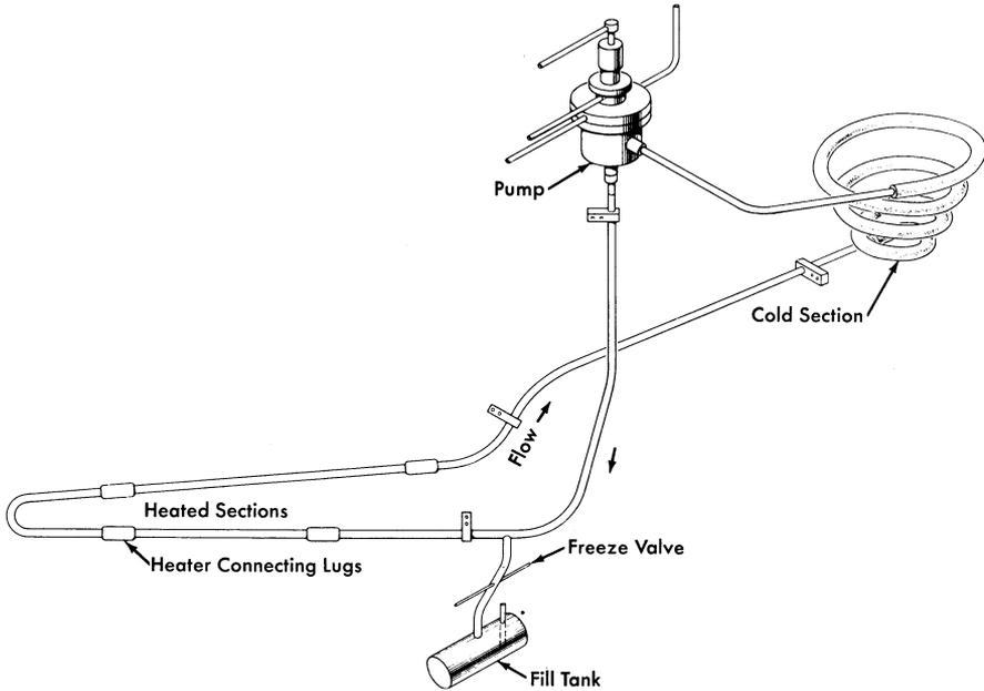
Fig. 13-2. Diagram of forced-circulation loop for corrosion testing.
