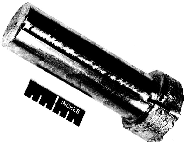
FIG. 13-9. Weld in slot of vacuum-melted ingot.
