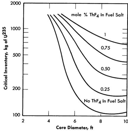
FIG. 14-3. Initial critical inventories of U<sup>235</sup> in two-region, homogeneous, molten fluoride-salt reactors. External fuel volume, 339 ft<sup>3</sup>.
