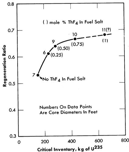
FIG. 14-5. Maximum initial regeneration ratios in two-region, homogeneous, molten fluoride-salt reactors fueled with  $U^{235}$ . Total power, 600 Mw (heat); external fuel volume, 339 ft<sup>3</sup>.
