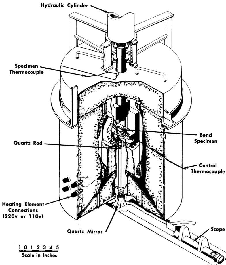
FIG. 13-10. Apparatus for bend tests at high temperatures.
