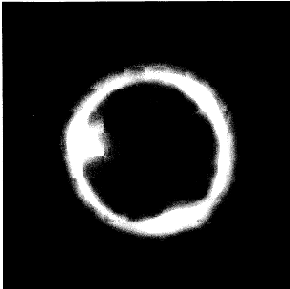
FIG. 22-2. In-pile capsule experiment with molten bismuth fuel, showing xenon and iodine diffusion into graphite.
