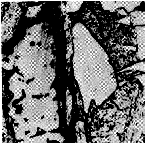
FIG. 21-6. Precipitation of Fe-Cr alloy in high-velocity cold-leg test section (HVL I-Run 1).
