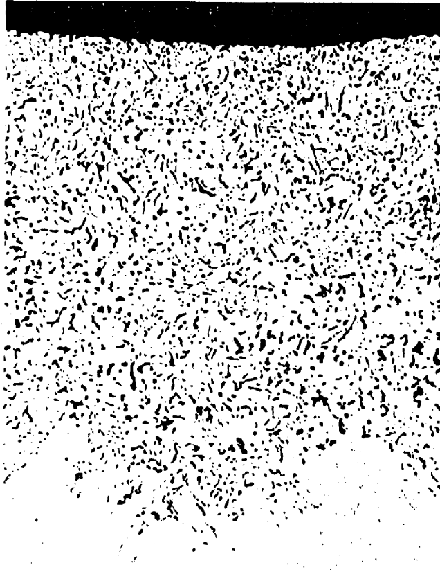
Figure 37 Photomicrograph of a sample of INCONEL 600 (20% Ni-15% Cr-5% Fe) after exposure to fluoride salt in a pumped loop for 15,000 hours at 1300°F. Voids near the surface are formed as chromium is removed selectively by the salt.
