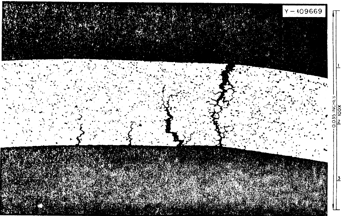
Fig. 25B. Photomicrograph of Hastelloy N tube burst specimen. Failure occurred after exposure to steam for 3.7 hr at 52,500 psi at 538°C. Steam was on the inside of the tube.
