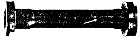
HASTELLOY N TUBE BURST SPECIMEN FAILED IN 3.7 hr IN STEAM AT 52,500 psi
