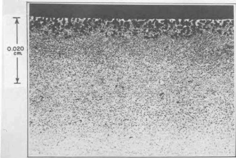
EFFECT OF GRAPHITE ADDITION ON LITHIUM CORROSION OF STAINLESS STEEL 1000°C FOR FORTY HOURS EXPOSED SURFACE AT TOP OF PHOTOMICROGRAPH
