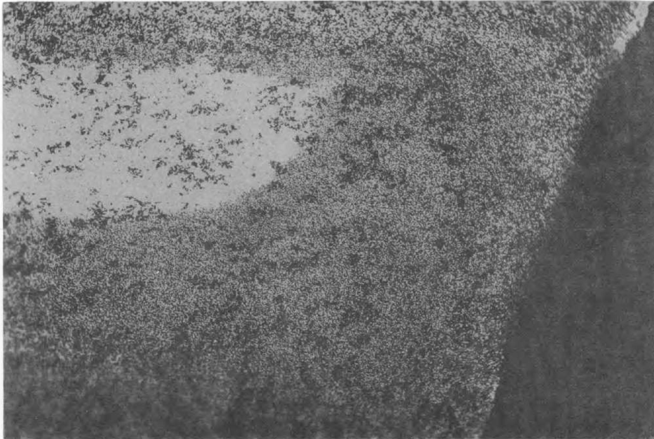
347 STAINLESS STEEL, SHOWING ATTACK AFTER 135 HOURS EXPOSURE TO LiF-U 4 EUTECTIC LIGHT SECTION IS UNATTACKED METAL
