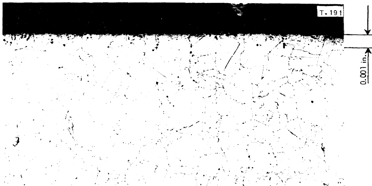
Fig. 10.17 - Corrosion of 316 Stainless Steel by Pretreated Fluoride Coolant. 250X. Specimen after 100 hr at 800°C in NaF-KF-BeF 2 eutectic; no appreciable attack. Compare with Fig. 10.6.
