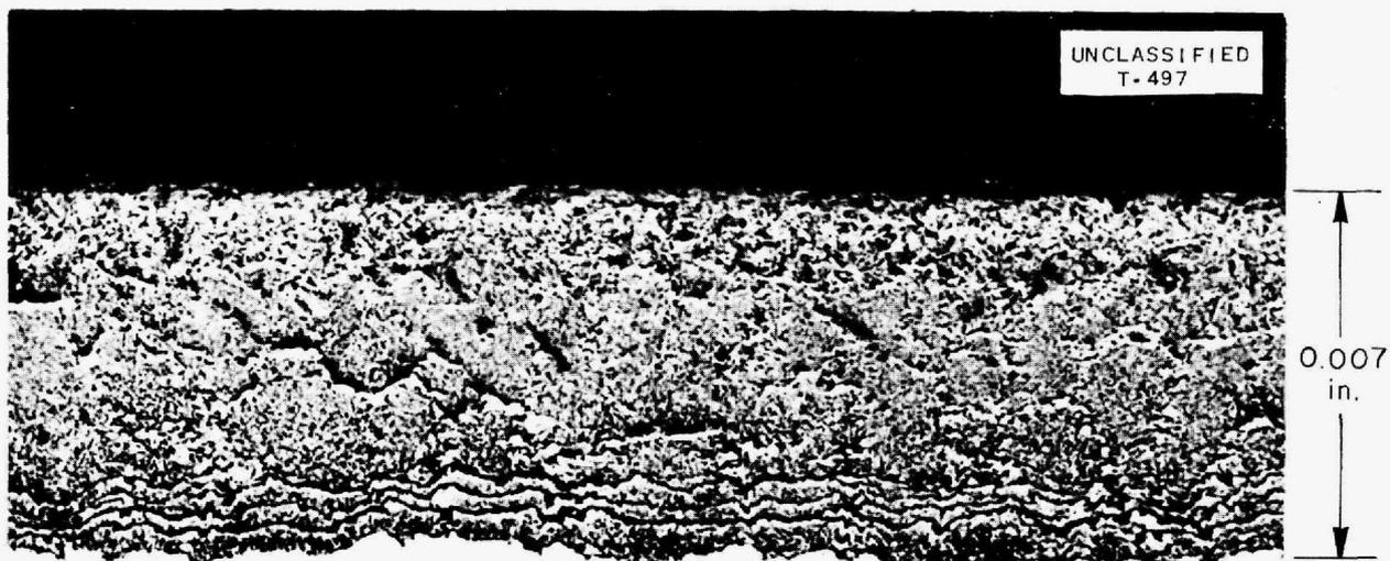
**Fig. 11.6. Surface of Inconel Specimen after 100 hr of Exposure to Lithium Hydroxide at 800°C.**
