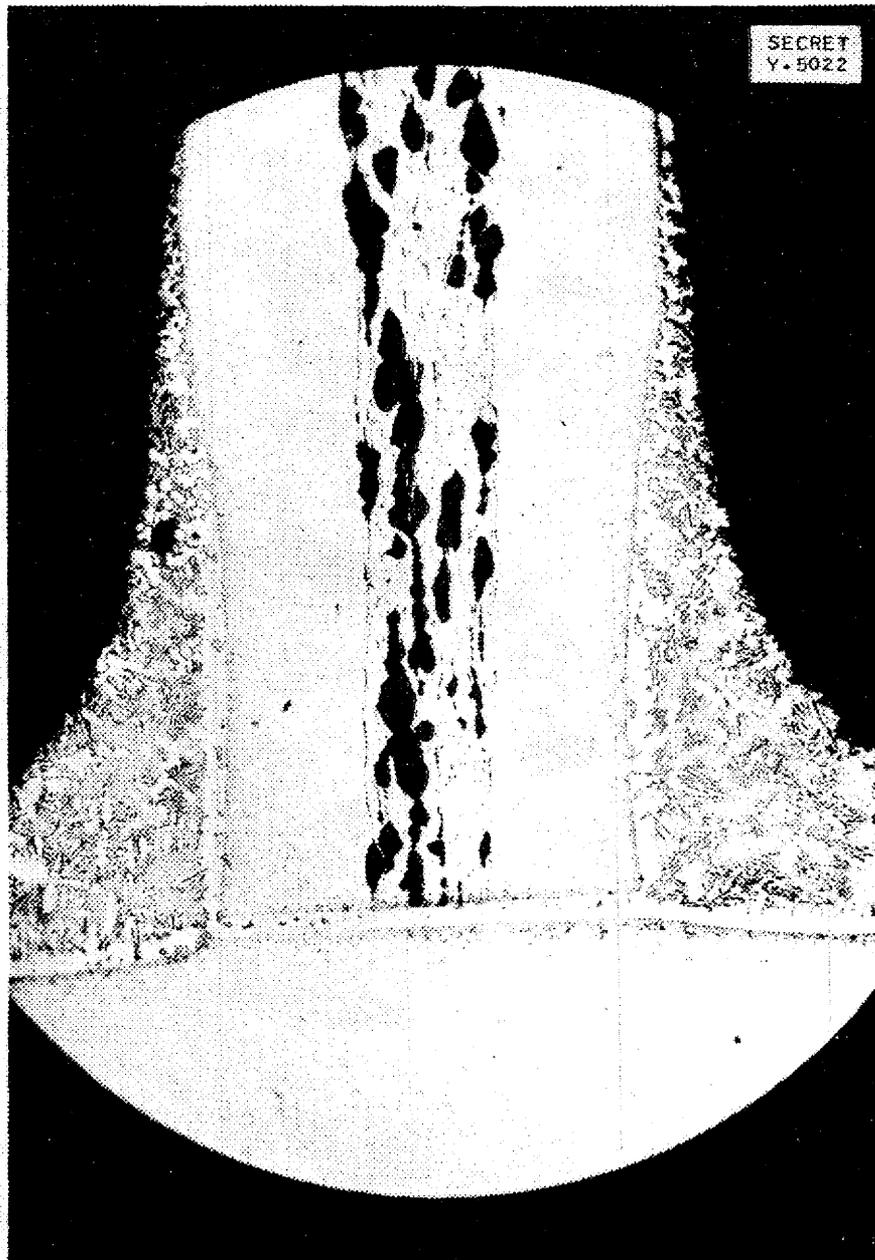
**Fig. 13.8. Transverse Section of a Stainless Steel—Clad Fuel-Element Butt Microbrazed to a Stainless Steel Sheet. Etchant, none. 40X.**
