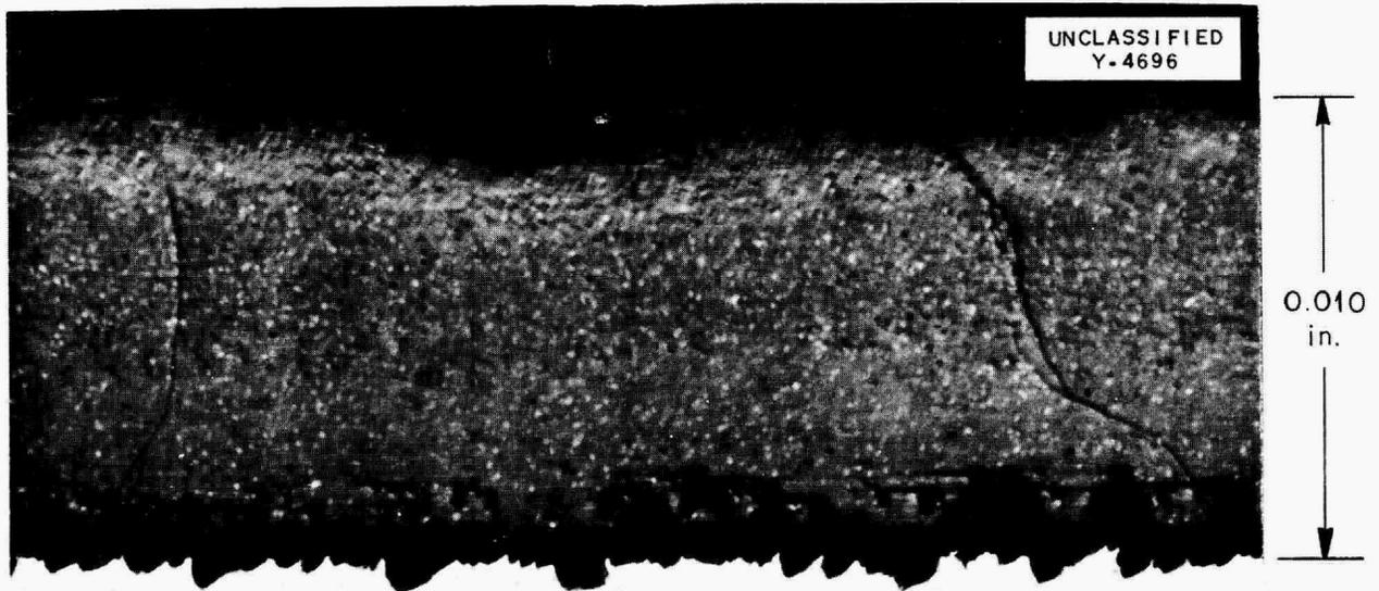
Fig. 11.1. Surface of 304 Stainless Steel after 100 hr of Exposure to Barium Hydroxide at 816°C.
