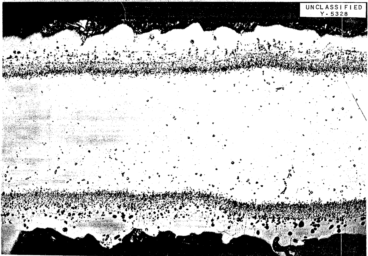
Fig. 34. Alloying Attack of Inconel Tested in 43% Tin-57% Bismuth Alloy for 100 hr at 1500°F. 100X.
