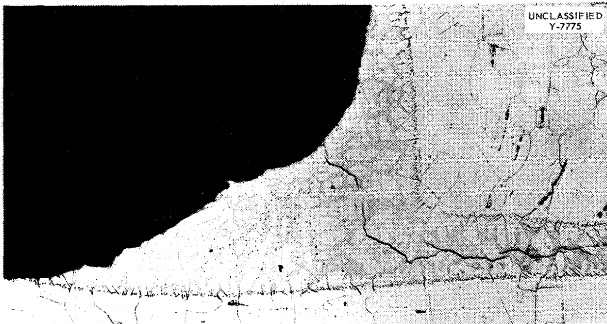
Fig. 12.8. Type 316 Stainless Steel Brazed with 16.5% Cr-10.0% Si-2.5% Mn-71.0% Ni After 100 hr at 1500°F in Sodium. Etched with aqua regia. 150X.
