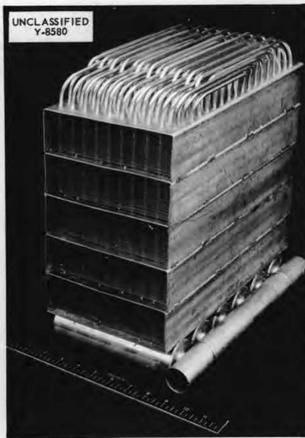
Fig. 11.2. Sodium-to-Air Radiator After Microbrazing.
