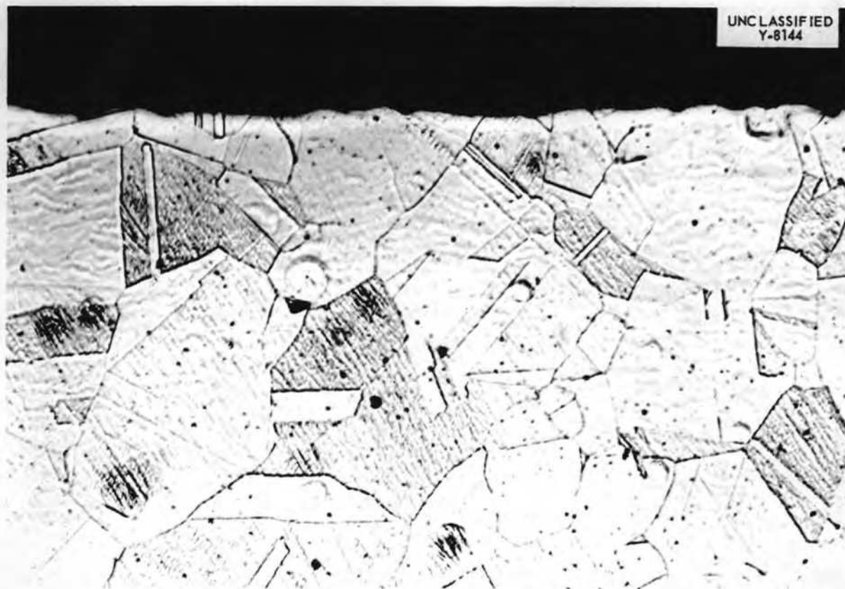
Fig. 10.5. Type 304 Stainless Steel After a Seesaw Test in a 5 wt % Na-95 wt % Pb Mixture for 100 hr at 830°C. 100X.
