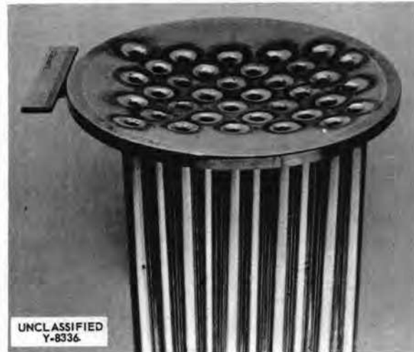
Fig. 11.1. An Experimental Heat Exchanger Subassembly After Cone-Arc Welding.
