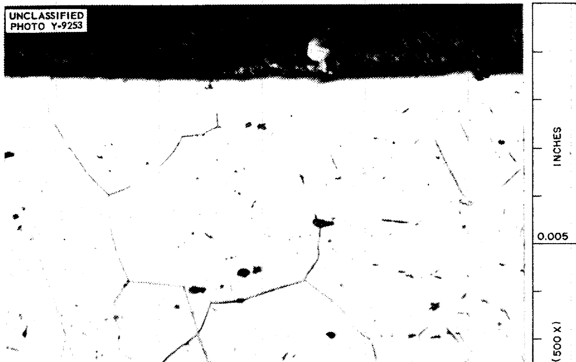
Fig. 7.10. Corrosion of Armco Iron by Lead in Quartz Thermal Convection Loop After 250 hr at 800°C. 500X
