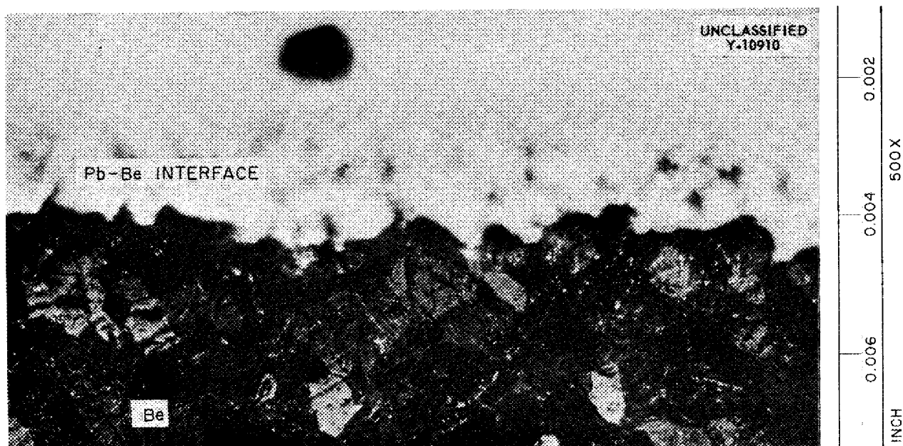
Fig. 6.8. Transverse Section of Beryllium Specimen Exposed to Liquid Lead at 815°C for 456 hr in the Hot Leg of a Quartz Thermal Convection Loop. Polarized light. 500X
