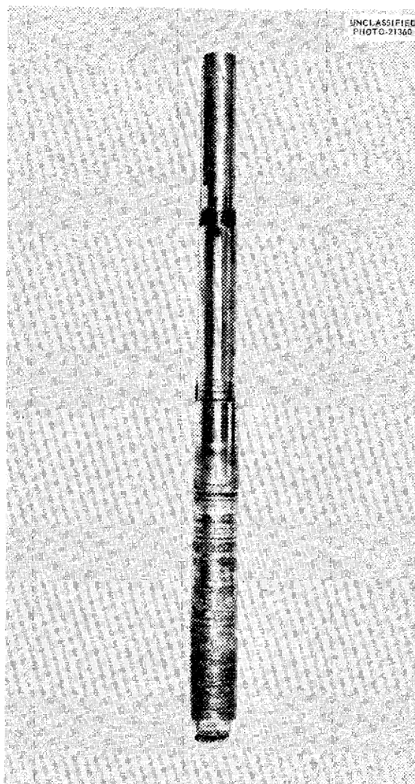
Fig. 2.10. Graphite-BeF 2 Packed Shaft After Continuous Operation for 4530 hr at Speeds of Up to 2500 rpm in Fluoride Mixture NaF-ZrF 4 -UF 4 (50-46-4 mole %).
