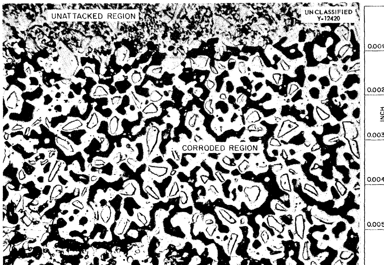
Fig. 5.13. Transverse Section of a Special Nonsigma-Phase Alloy (16% Ni-37% Cr-47% Fe) Specimen from the Hot Leg of a Quartz Thermal-Convection Loop Which Circulated Liquid Lead. 750X.
