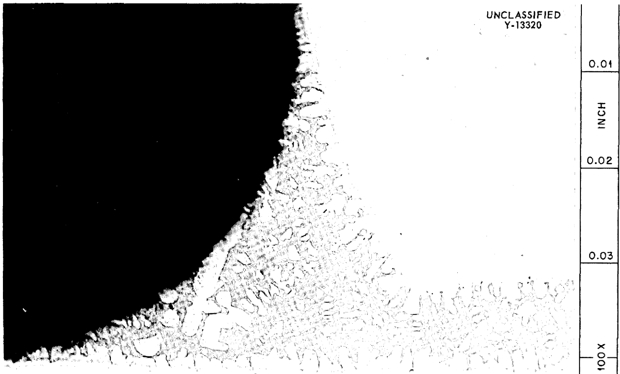
Fig. 7.31. Inconel T-Joint Brazed with G-E Brazing Alloy No. 81 and Tested in Static Air for 500 hr at 1500°F. Note negligible attack. Etched with electrolytic oxalic acid. 100X.
