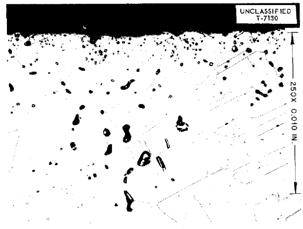
Fig. 6.5. Hot Leg of Forced-Circulation Inconel Loop 4690 After Circulating NaF-ZrF 4 -UF 4 . 250X. Reduced 31%.
