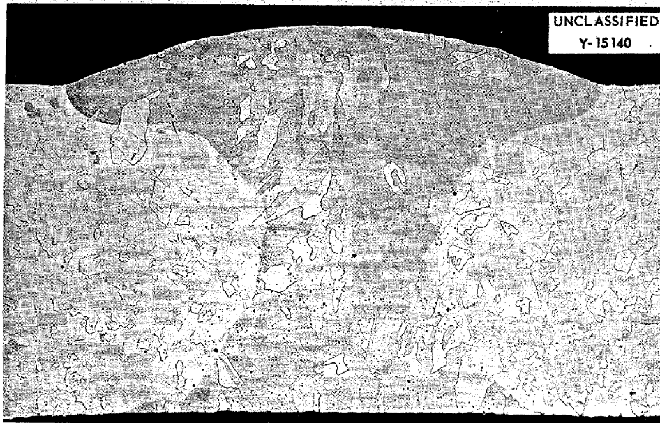
Fig. 10.2. Cross Section of Welded "L" Nickel Test Coupon Exposed to Molten Salt in a Nickel Reaction Vessel. Note uniformity of attack. Etched with KCN plus (\text{NH}_4)_2\text{S}_2\text{O}_8 . 12X.
