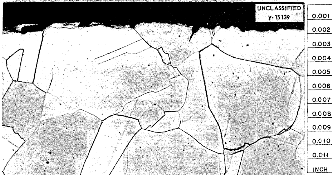
Fig. 10.4. Inner Surface of Specimen of "A" Nickel Reaction Vessel Taken from Region Exposed to ARE-Type Fuel. Note nonuniform surface attack. Etched with KCN plus (\text{NH}_4)_2\text{S}_2\text{O}_8 . 250X.
