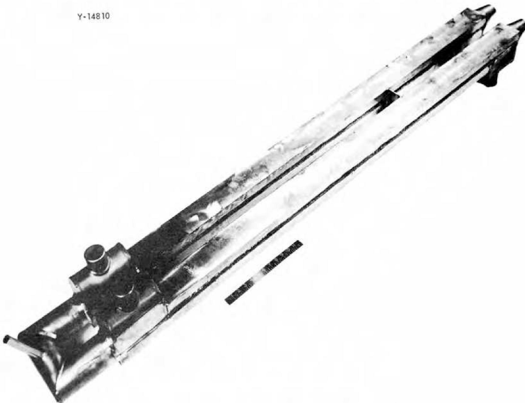
Fig. 16. A Completed 1-Mw Heat Exchanger.
