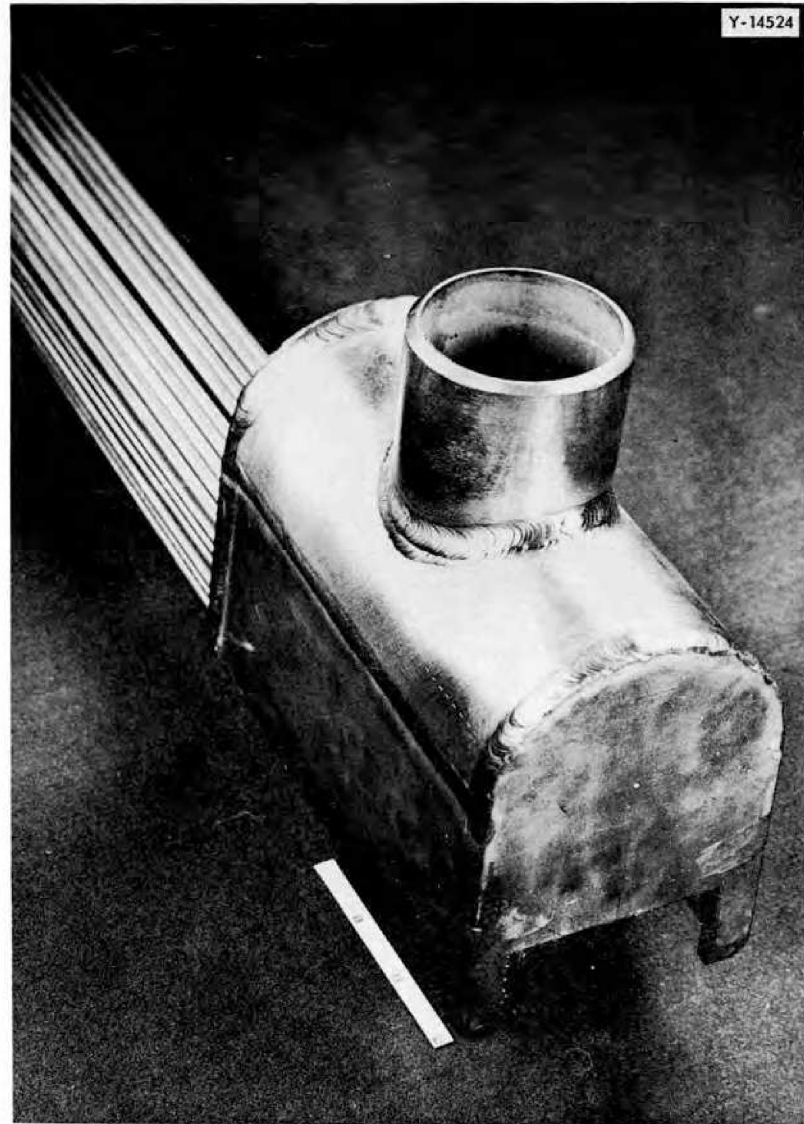
Fig. 10. A Completed Leaktight Header Section.
