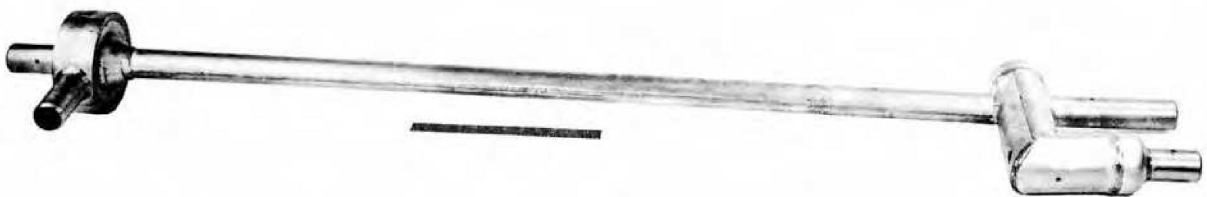
Fig. 31. The Completed 20-Tube High-Velocity Heat Exchanger.
