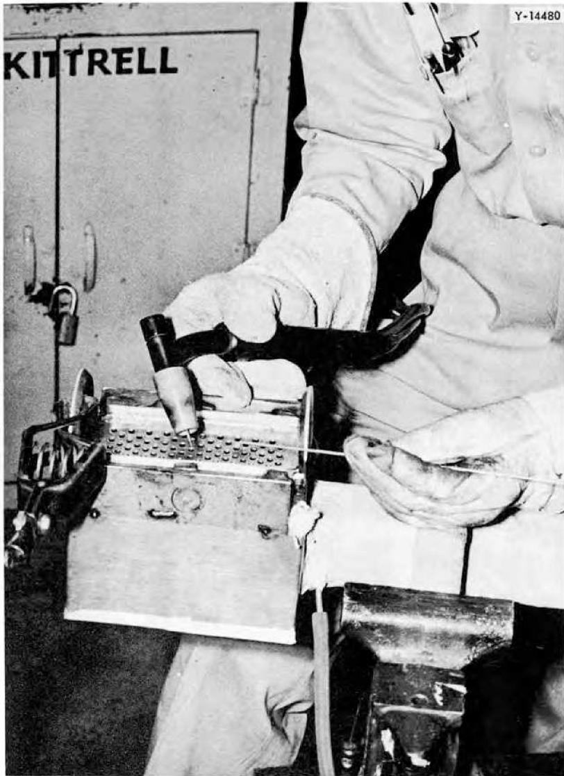
Fig. 9. Header in Early Stages of Fabrication.
