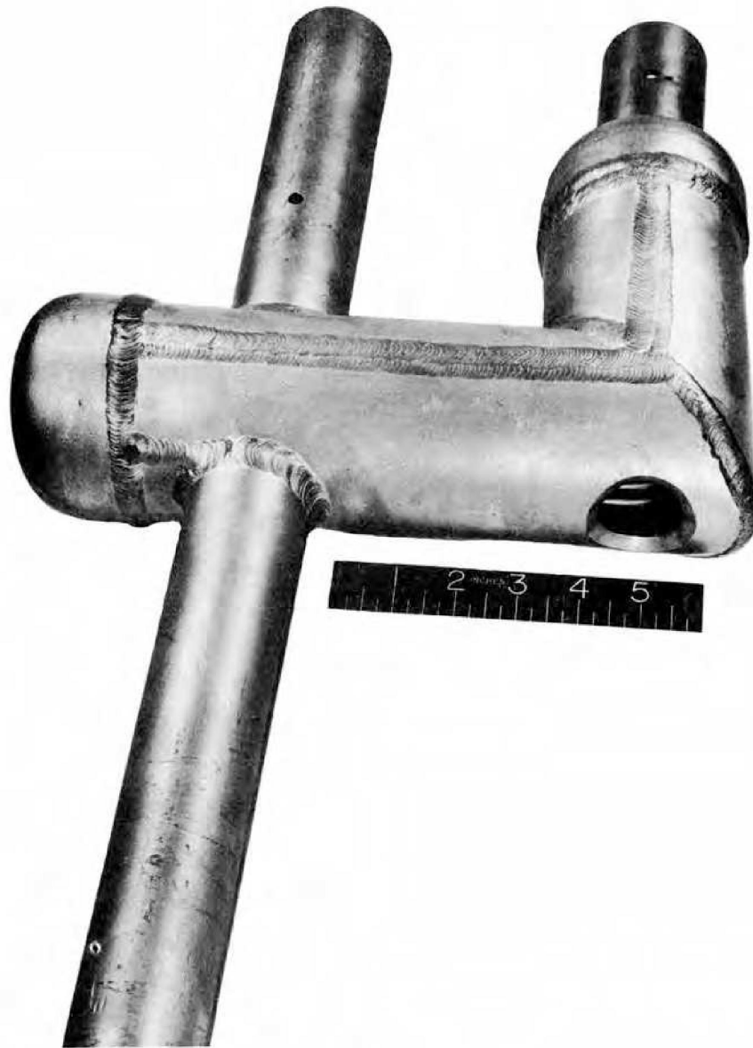
Fig. 30. The NaK Inlet End of a 20-Tube Heat Exchanger. Note the "window" through which the brazing alloy was preplaced and inspected.
