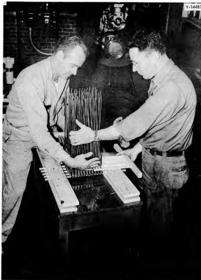
Fig. 24. Fin Assembly in Early Stages of Fabrication. It can be seen that the process was difficult even with the use of precision jigs.
