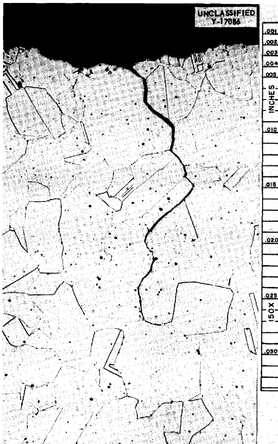
Fig. 5.23. Wall of Condenser Pipe of Inconel—Boiling-Sodium Loop Operated for 1000 hr. Temperature at location shown was between 1150 and 1325°F.
