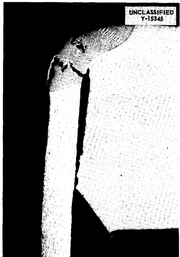
Fig. 6.11. Tube-to-Header Weld Showing Severe Cracks. Etched with oxalic acid. 21X.
