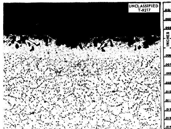
Fig. 5.7. Maximum Hot-Leg Attack Found in Hastelloy B Thermal-Convection Loop 816 Operated with NaF-KF-LiF-UF 4 (11.2-41-45.3-2.5 mole %) as the Circulated Fluid. 250X. Reduced 32%. (Secret with caption)
