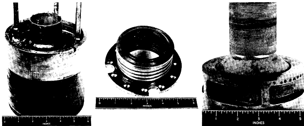
Fig. 2.5. Disassembled ART Fuel Pump (Model MF-2), Showing Greasy Material That Formed When Leakage Oil Contacted the Vapors from the NaK Being Circulated in the Pump at 1400°F. This pump operated continuously for 2056 hr before disassembly.
