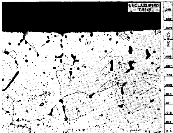
Fig. 5.11. Maximum Hot-Leg Attack Found in Inconel Thermal-Convection Loop 840 Which Circulated \text{RbF-ZrF}_4\text{-UF}_4 (50-46-4 mole %) for 500 hr at a Hot-Leg Temperature of 1500^\circ\text{F} . 250X. Reduced 32%. (Caption with caption)
