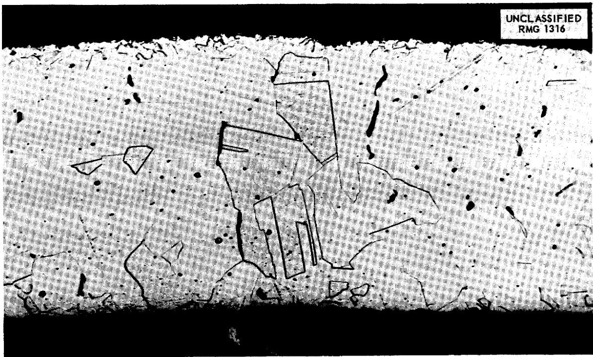
Fig. 8.10. Structure Near Fracture in Inconel Out-of-Pile Tube-Burst Specimen That Was Internally Pressurized with Helium to a Fiber Stress of 2000 psi and Ruptured After 356 hr at 1500°F. 300X.
