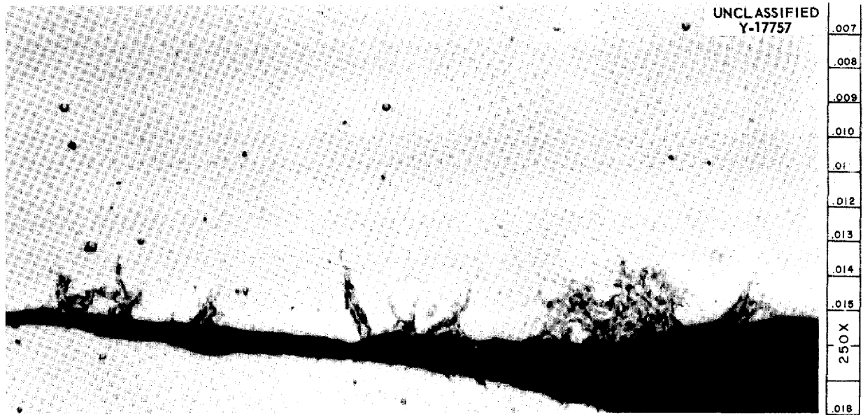
Fig. 5.24. Hot Zone of Inconel Thermal-Convection Loop 863 Which Circulated Sodium Hydroxide for 100 hr. The wall temperature near this point was 1180°F; the fluid temperature was 1120°F; the cover gas was hydrogen. 250X.
