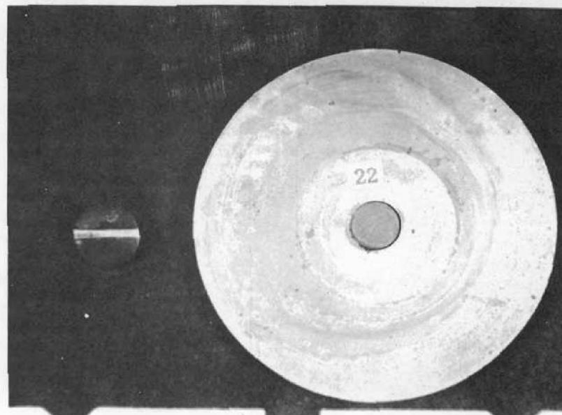
Test No. 22. Pin: Carboloy 608, \text{Cr}_3\text{C}_2 Plate: Adamas Grade A, WC
