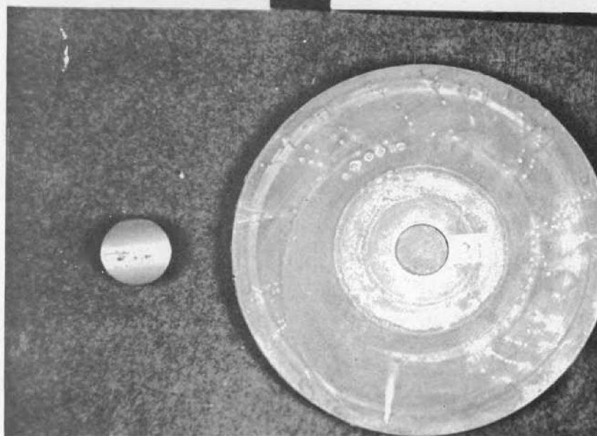
Test No. 24. Pin: Adamas Grade A, WC Plate: Kennametal 138A, TiC + Co
