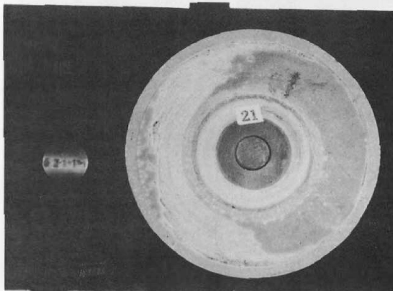
Test No. 21. Pin: Adamas Grade A, WC Plate: Adamas Grade A, WC
