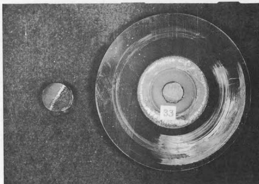
Test No. 33. Pin: Carboloy 608, \text{Cr}_3\text{C}_2 Plate: Norton Norbide, \text{B}_4\text{C}
