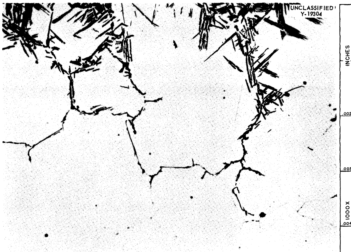
Fig. 3. Intergranular Attack at Bottom of Corrosion-Product Layer Shown in Fig. 1. Some transgranular attack can also be noted. Unetched. 1000X.
