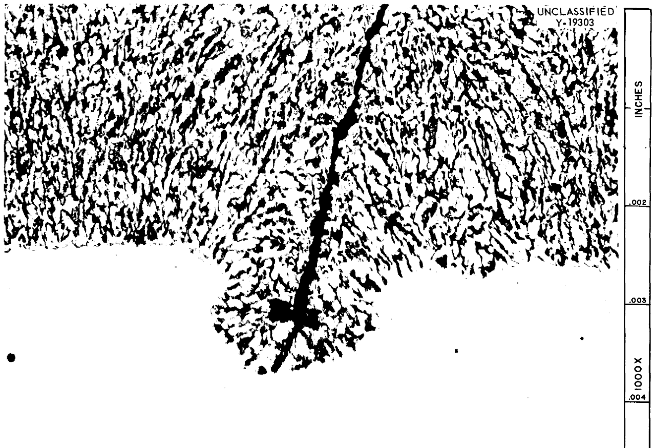
Fig. 5. Network of Nonmetallic Particles Near Bottom of Corrosion-Product Layer Formed on 80% Fe-20% Cr Alloy. Unetched. 1000X.
