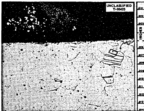
Fig. 3.1.4. Deposits Found in Inconel Forced-Circulation Loop 7426-11 Which Circulated Sodium at a Maximum Temperature of 1350°F for 1000 hr. 250X. Reduced 32%. (Confidential with caption)
