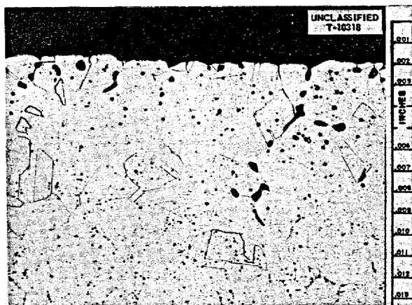
Fig. 3.1.1. Hot-Leg Surface of Inconel Forced-Circulation Loop 7425-14 After Operation with the Fuel Mixture (No. 70) NaF-ZrF 4 -UF 4 (56-39-5 mole %) for 1000 hr at a Maximum Fuel Temperature of 1525°F. 250X. Reduced 34%. (Secret with caption)
