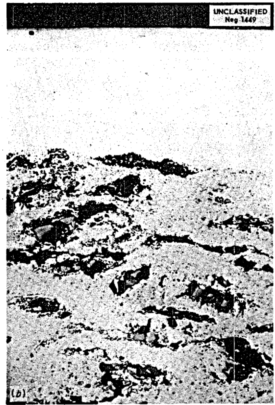
Fig. 4.2.28. Type 304 Stainless Steel Clad CaB 6 -Fe Cermet Before and After Irradiation in the LITR to a Thermal-Neutron Dose of 5.2 \times 10^{19} nvt. (a) Unirradiated. (b) Irradiated. 250X. Reduced 27%.
