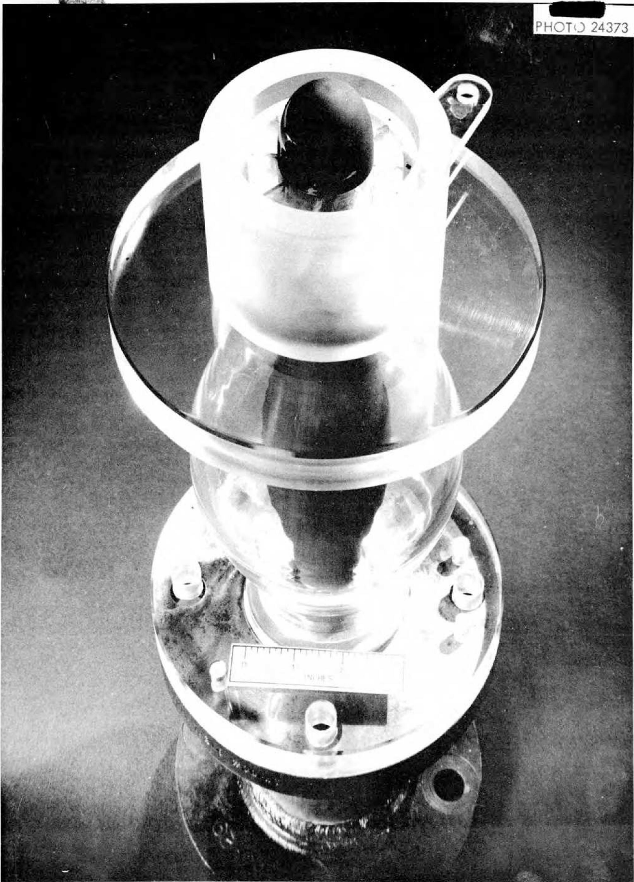
Fig. 30. '21-Inch' ART Core Model with Turning-Vane Section at the Inlet.
