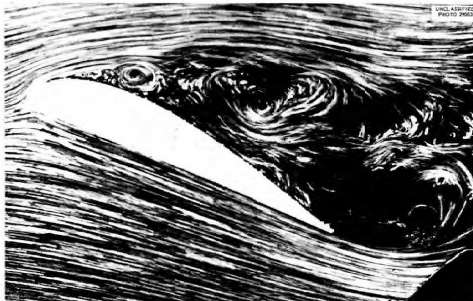
Fig. 66. Visualization of Flow in a Separation Region Behind an Aerofoil. (Reference 30)
