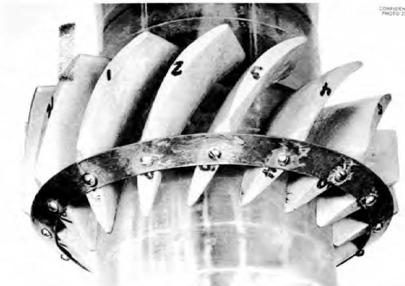
Fig. 65. GS-2 Guide Vanes and Baffle Plate Mounted on Inner Wall of the 24-inch ART Core at the Inlet. (Reference 29)
