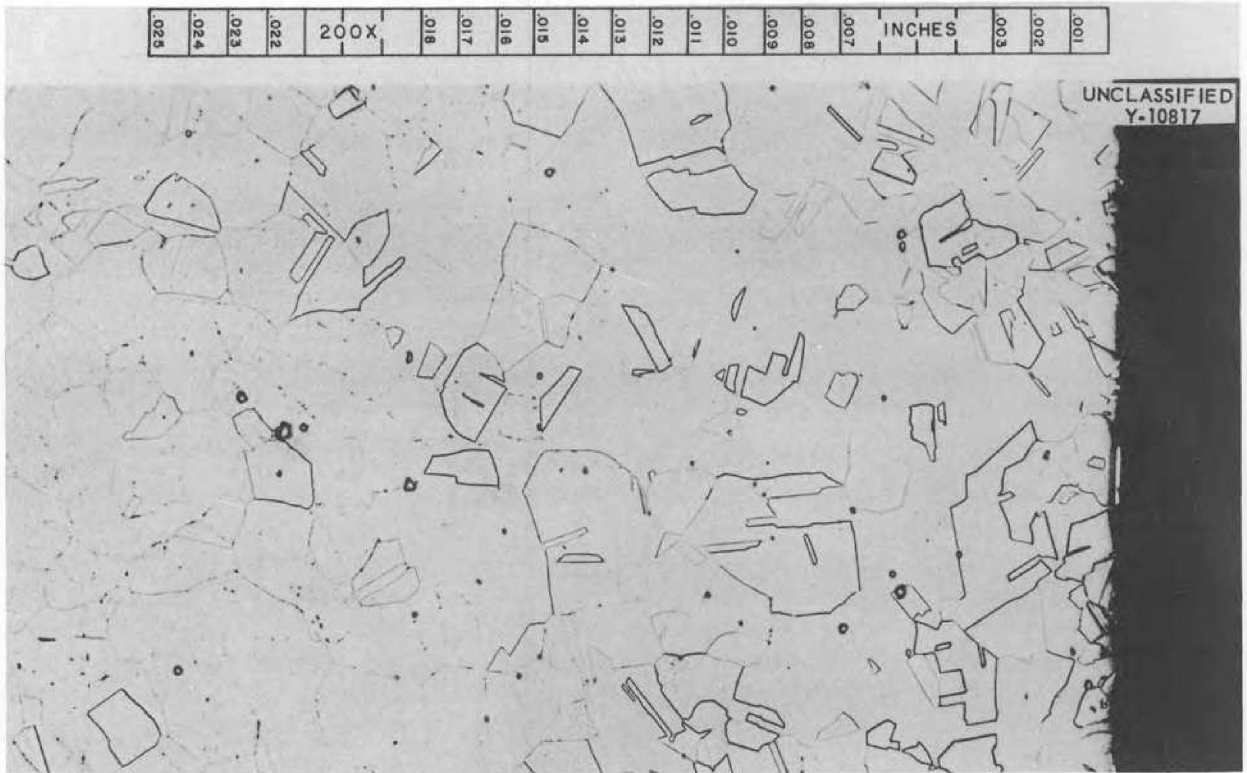
Fig. 65. Photomicrograph of As-Received Inconel Tested at 1500°F Under 3500-psi Stress in Sodium. 200X. Electrolytically etched with 10% oxalic acid.
