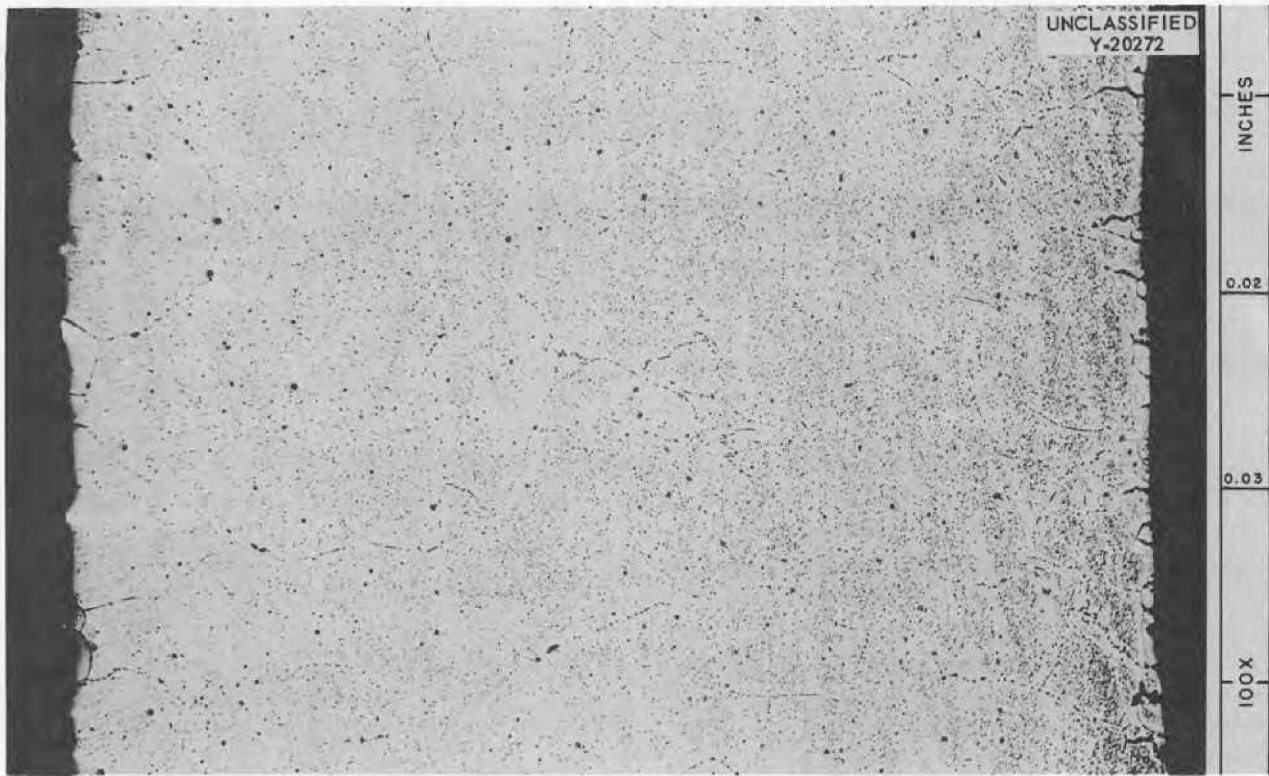
Fig. 77. Photomicrograph from Inconel Tube-Burst Specimen Tested in Argon at 1500°F Under 4000-psi Stress. 100X. Electrolytically etched with 10% oxalic acid.
