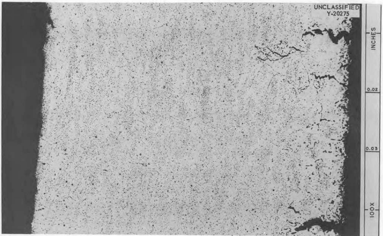
Fig. 79. Photomicrograph from Inconel Tube-Burst Specimen Tested in Fused Salt No. 30 at 1500°F Under 5000-psi Stress. 100X. Electrolytically etched with 10% oxalic acid. (Secret with caption)
