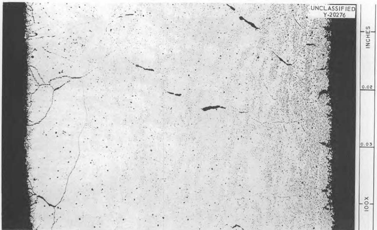
Fig. 76. Photomicrograph from Inconel Tube-Burst Specimen Tested in Argon at 1500°F Under 5000-psi Stress, 100X. Electrolytically etched with 10% oxalic acid.
