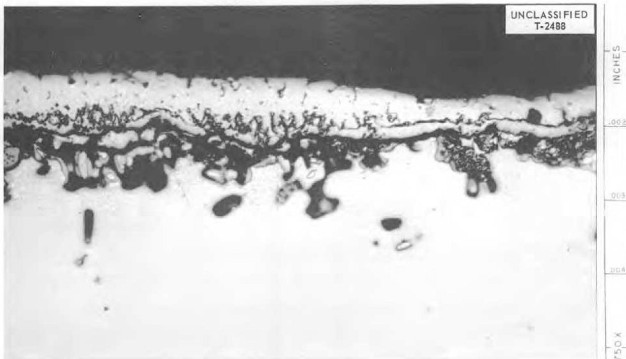
Fig. 11. Hot Leg of Inconel Loop After Circulating Molten Fluorides with Small Addition of Titanium Hydride. 750X. (Secret with caption)
