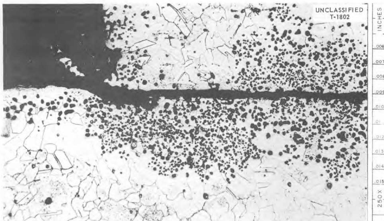
Fig. 13. Increase in Attack in a Crevice of an Inconel Loop. 250X.
