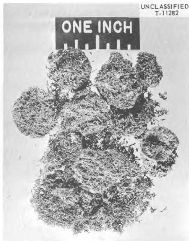
Fig. 24. Metal Deposit Taken from Cold Leg of an Izett Iron Loop.
