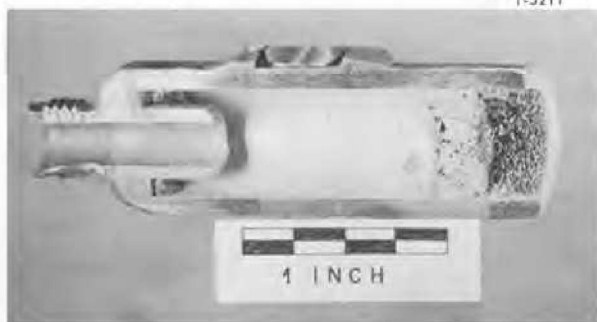
Fig. 8. Metallic Deposit Found at Top of Cold Trap from Loop 344.
