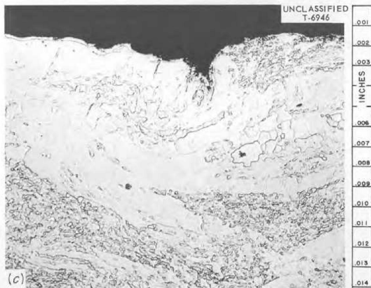
Fig. 27. Effect of Operating Time on Corrosion of Molybdenum by Fluoride 30. (a) As received; (b) 250 hr; (c) 1000 hr; (d) 2000 hr. 250X. Reduced 17%.
