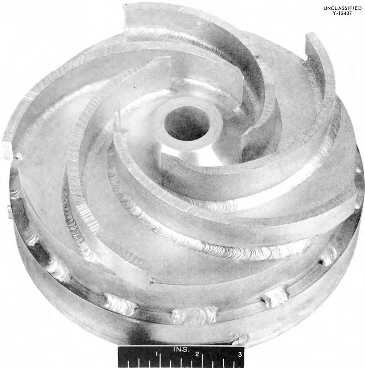
Fig. 27. Impeller After Hellarc Welding of Vanes to Drive-Shaft Hub. Impeller is tack-welded to a carbon steel strong-back.
