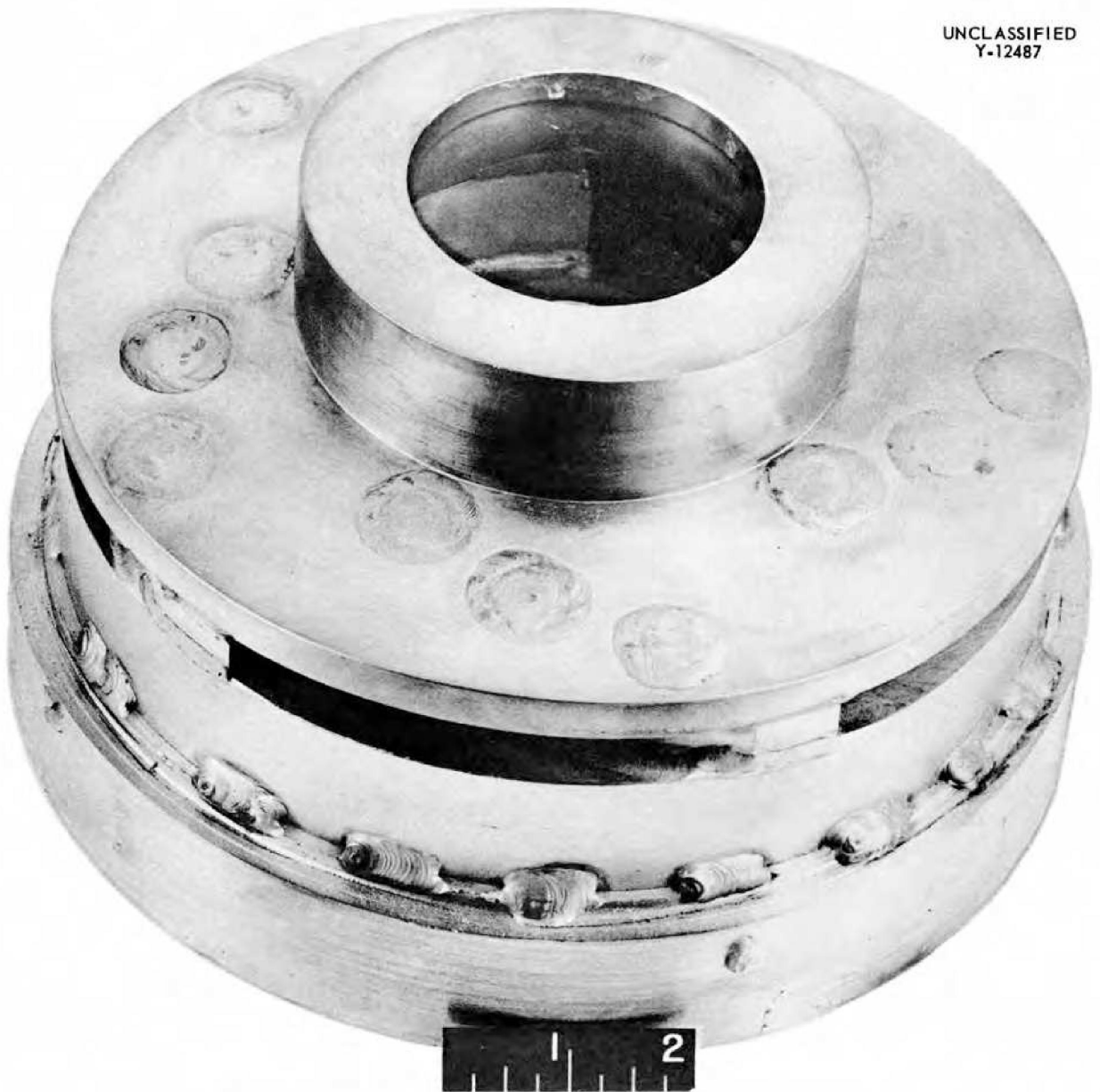
Fig. 28. Impeller with Fluid-Entrance Hub Plug-Welded into Position.
