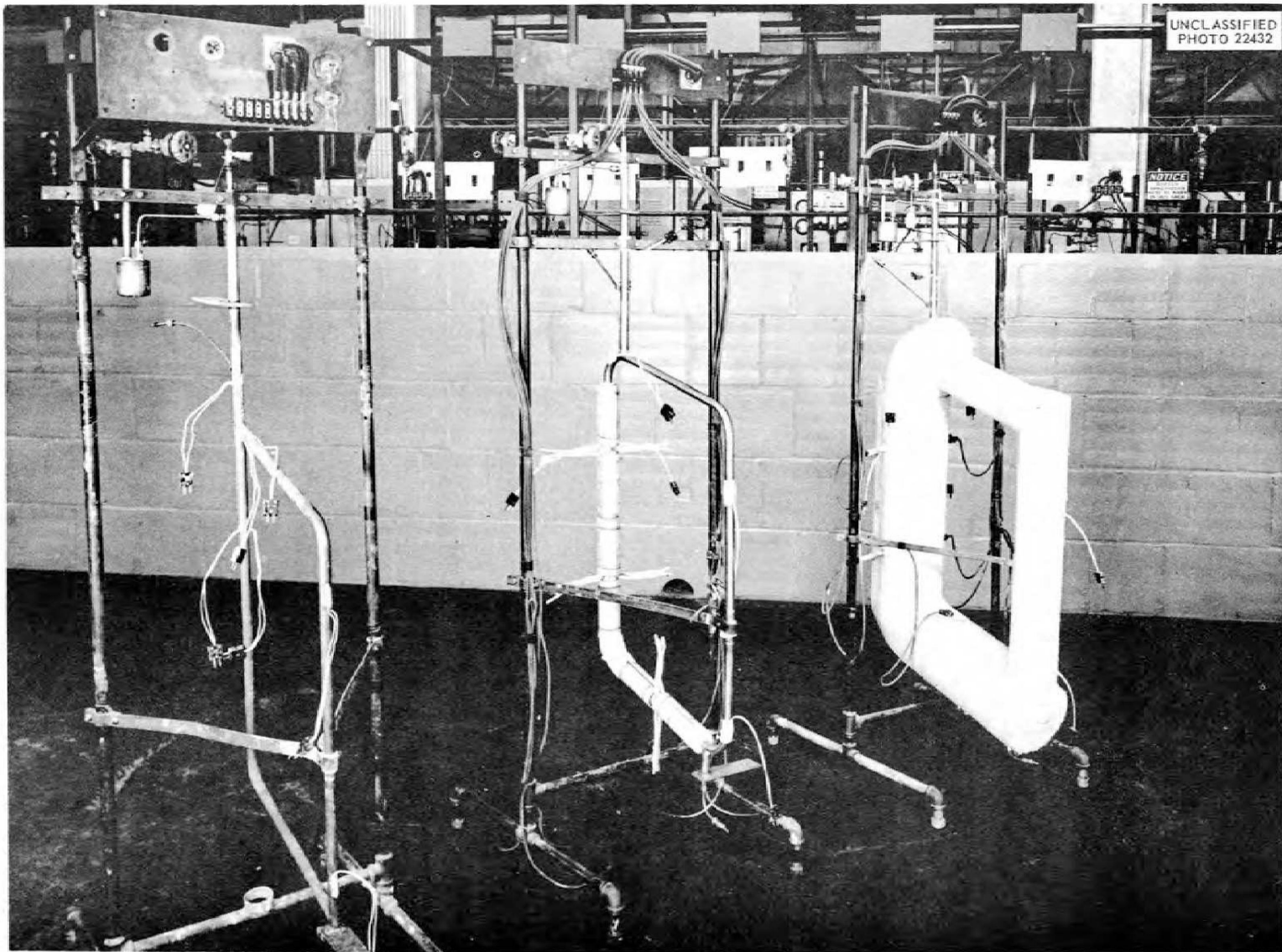
Fig. 6. Natural-Convection Corrosion Test Loops.
