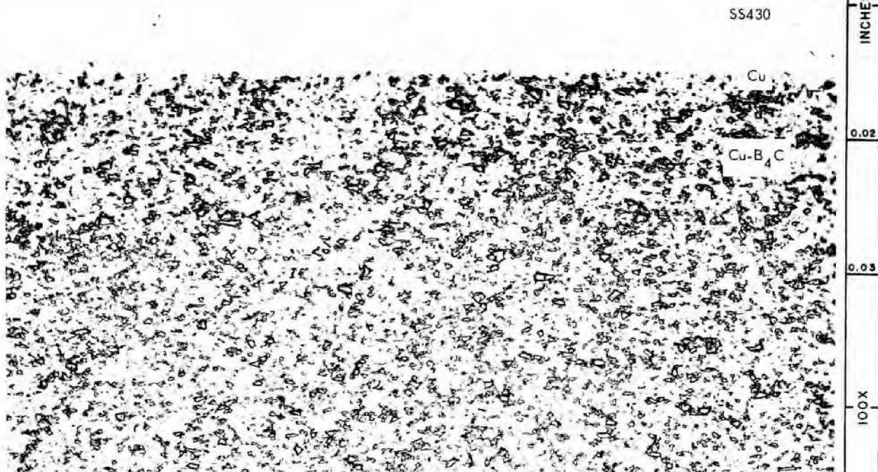
Fig. 9. Microstructure of Neutron-Shield Material. 100X.
