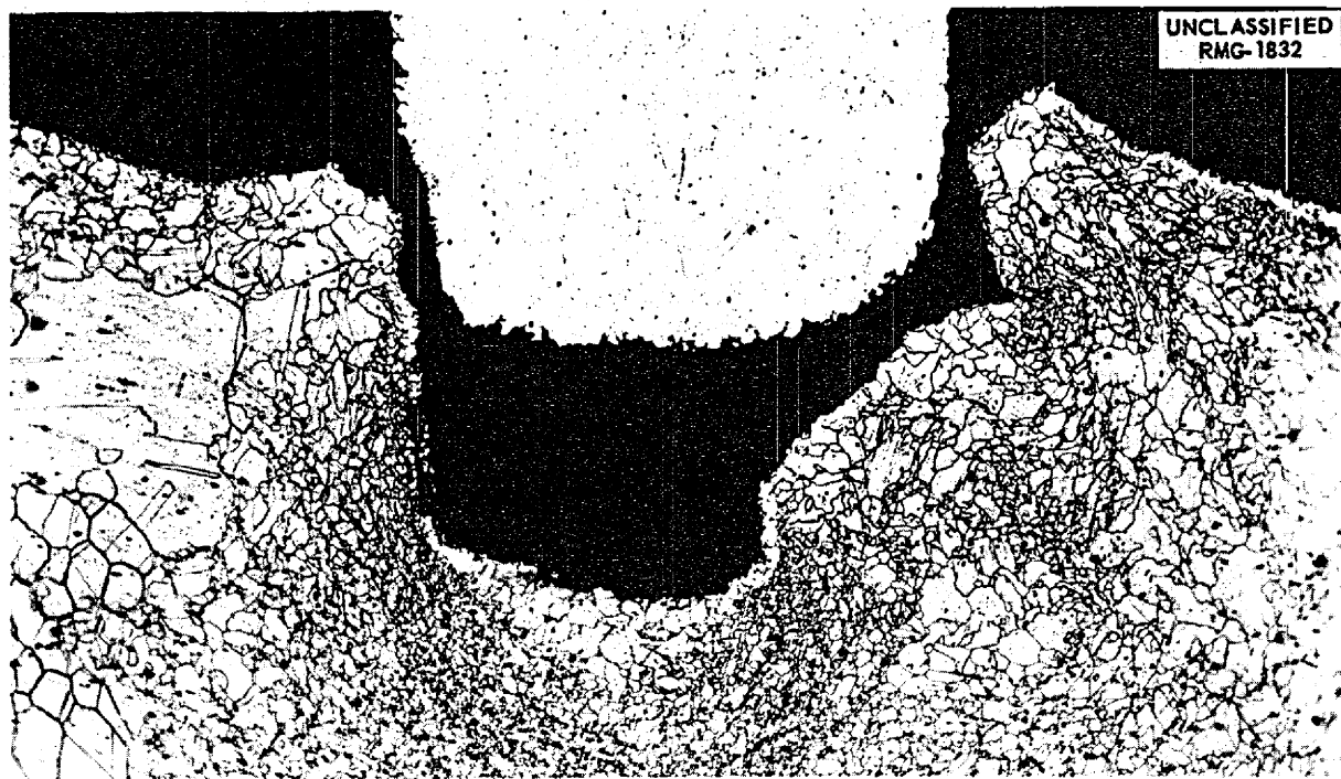
Fig. 4.1.16. Section of Specimen F5 Showing Fin-to-Tube Wall Junction in ARE Fuel-to-Helium Heat Exchanger. Fins were wound helically in grooves and were not brazed to the tubes. Etched. 100X. ( Secret with caption )
