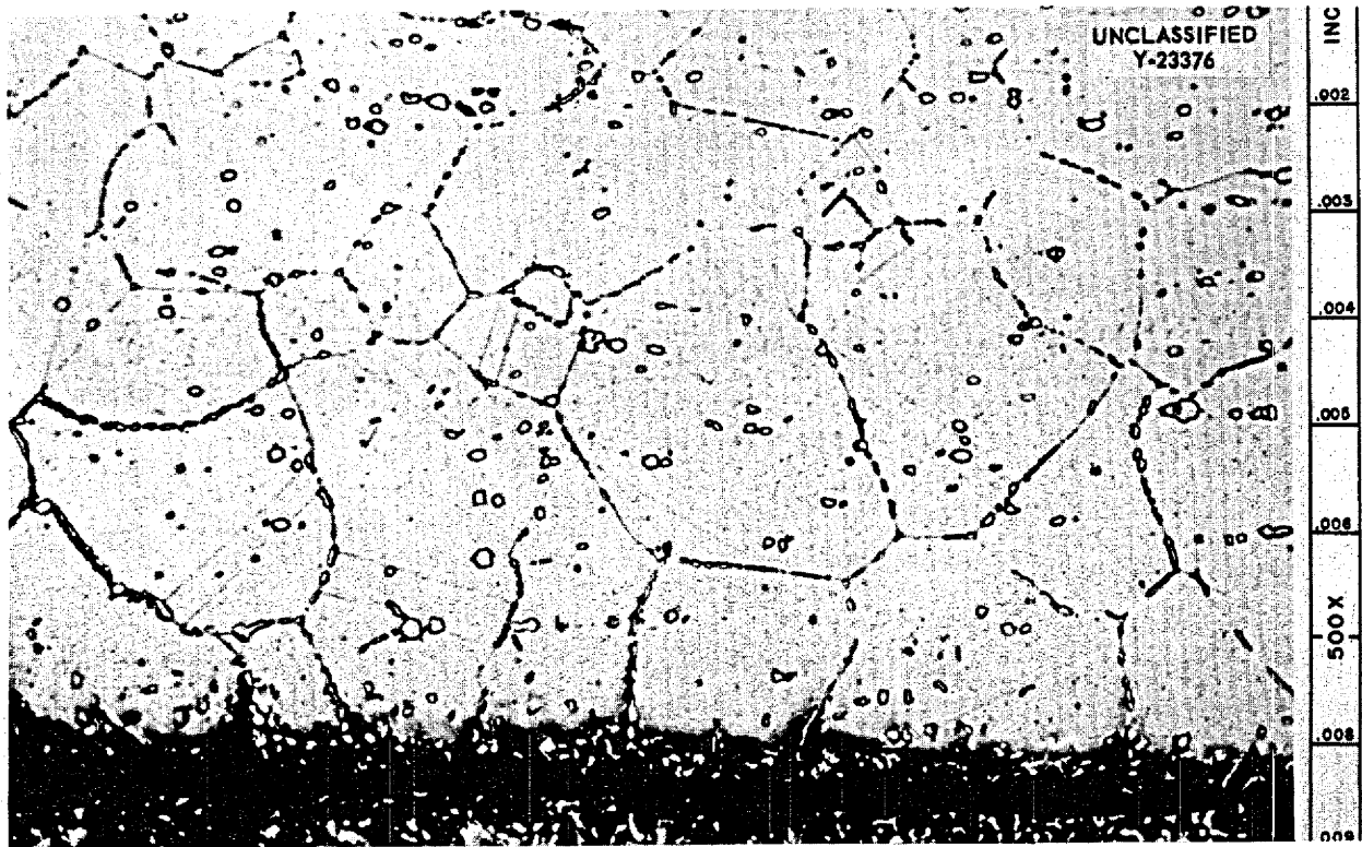
Fig. 3.1.5. Specimen of Alloy 30-62 Tested in the Annealed and Aged Condition at 8000 psi and 1500°F in Fuel 107. Etchant: chrome regia. 500X. (Secret with caption)
