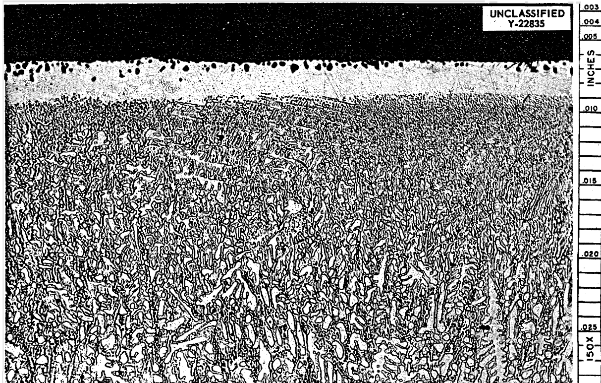
Fig. 3.2.24. Coast Metals Brazing Alloy No. 52 (89% Ni-5% Si-4% B-2% Fe) After Exposure for 100 hr at 1500°F to NaF-KF-LiF-UF 4 (11.2-41-45.3-2.5 mole %, fuel 107) in a Seesaw Furnace Apparatus. Etchant: 10% oxalic acid, electrolytic. 150X. ( Secret with caption )
