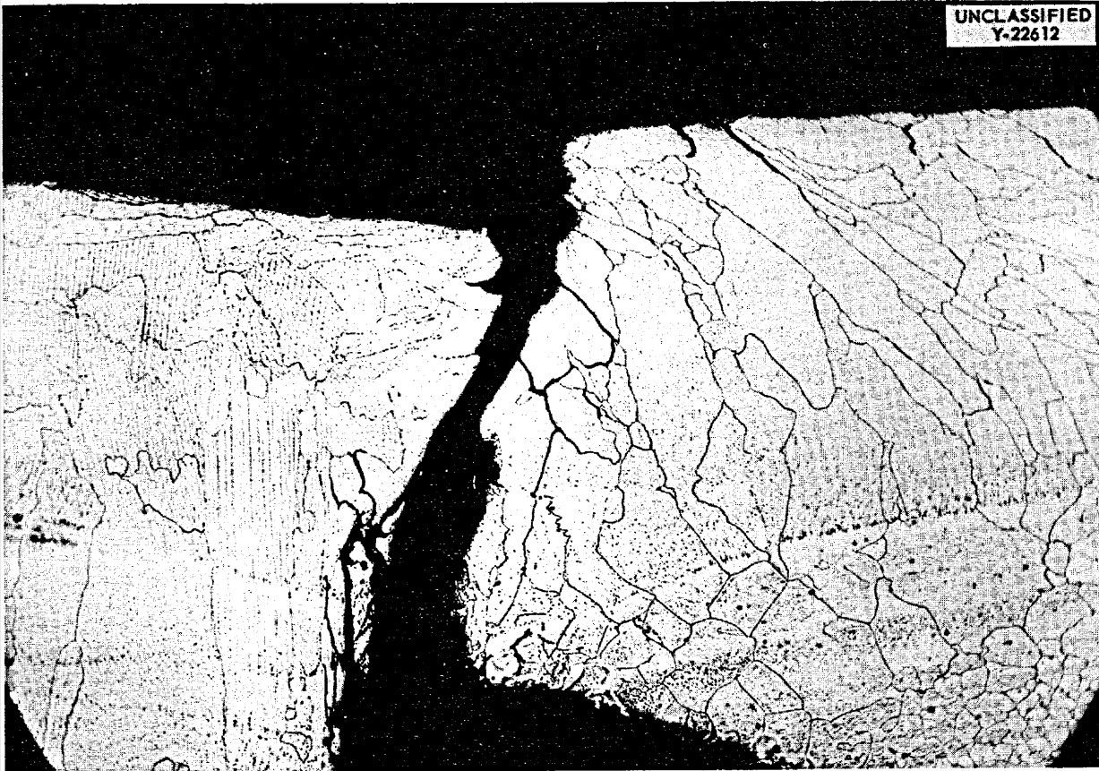
Fig. 3.3.2. Photomicrograph of Weld Fracture Shown in Fig. 3.3.1. 100X. Etchant: electrolytic oxalic acid.
