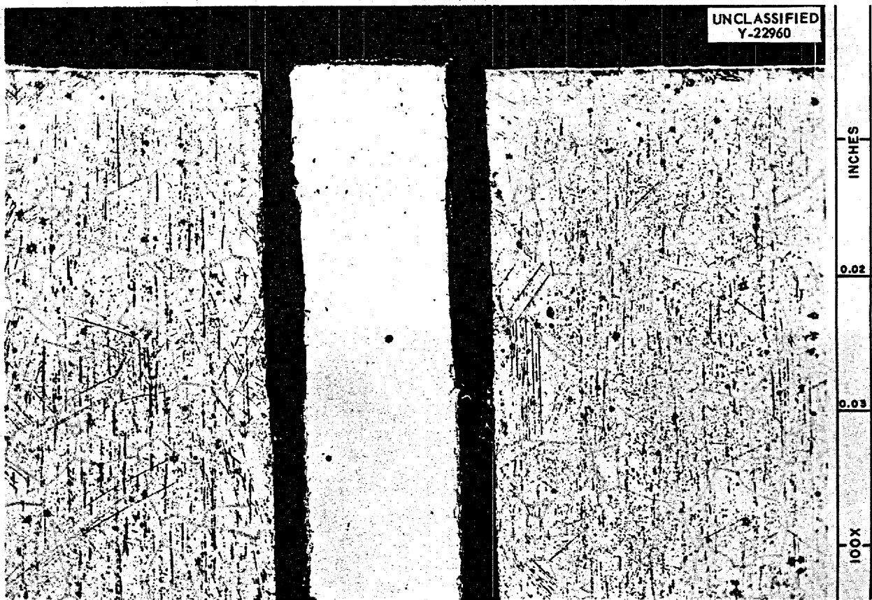
Fig. 1.7.7. Photomicrograph of End of "Gunbarrel" Thermocouple After 300 hr of Exposure to Static NaF-ZrF 4 -UF 4 (50-46-4 mole %) at 1200°F. Note the absence of the nickel plate between the end of the central nickel wire and the Inconel on either side. (Secret with exception)
