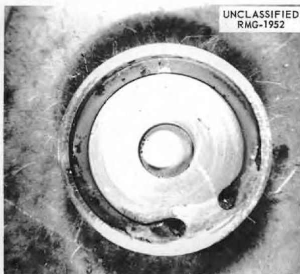
Fig. 4.1.8. Cover Plate of Housing for Impeller of Pump Used in MTR In-Pile Loop No. 6. \frac{1}{2}X .
