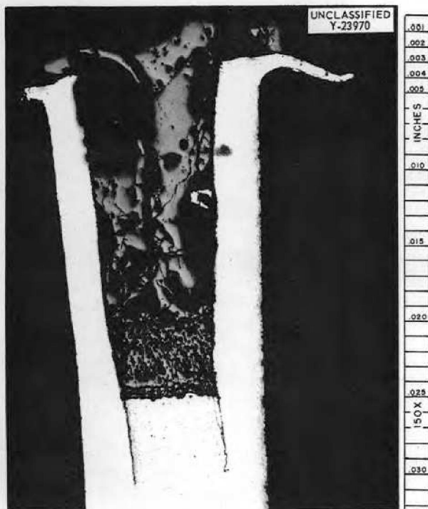
Fig. 3.6.9. Stainless-Steel-Clad Copper Fin with Unprotected Edge Showing Oxidation That Occurred During Operation of ART Prototype Radiator No. 1. Unetched. 150X. Reduced 24.5%. (Secret with caption)
