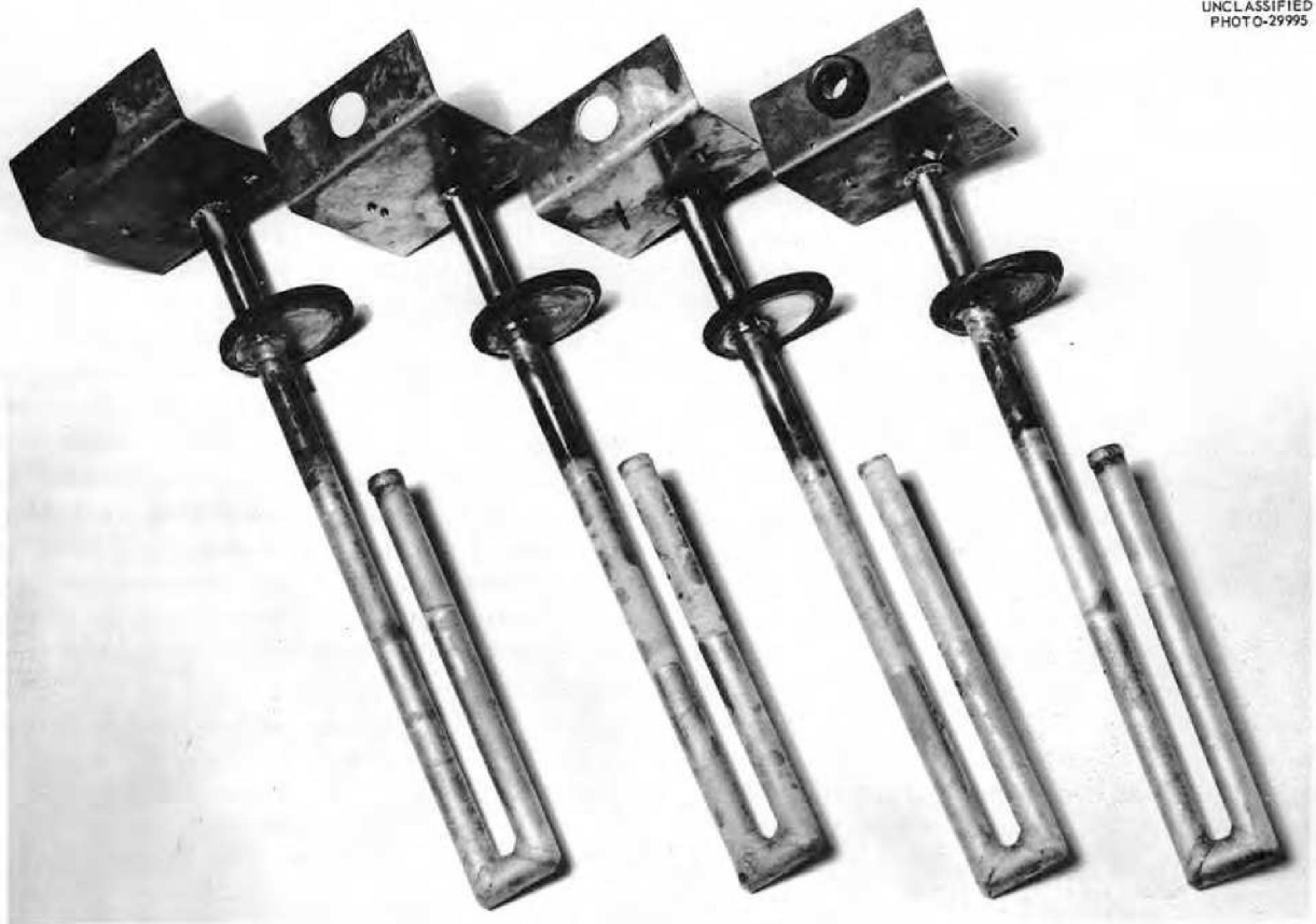
Fig. 1.3.14. Liquid-Metal-Level Transducers That Were Installed in a Life-Testing Facility After Having Operated for 3480 or 2440 hr.
