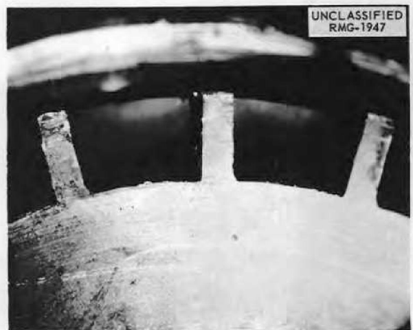
Fig. 4.1.3. Teeth of Impeller from Pump Used in MTR In-Pile Loop No. 6. 4X. Reduced 11%.
