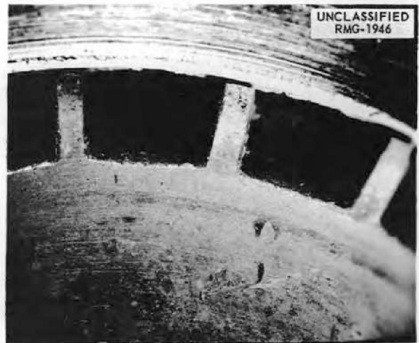
Fig. 4.1.2. Teeth of Impeller from Pump Used in MTR In-Pile Loop No. 5. 4X. Reduced 11%.
