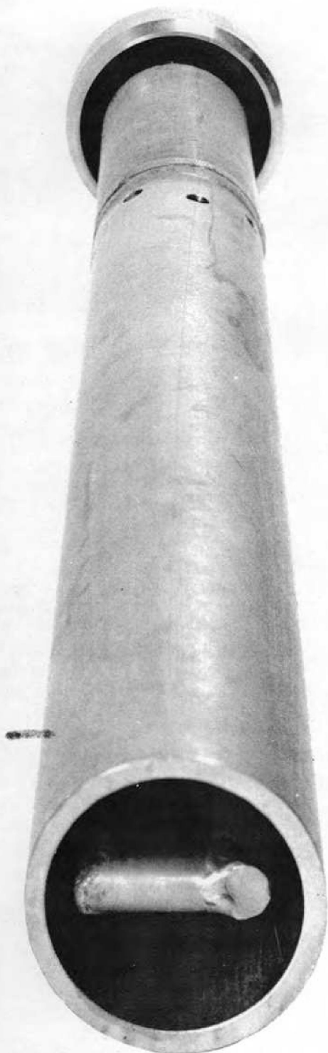
Fig. 1.3.9. Assembled Resistance-Type Fuel Level Probe. (Secret with caption)
