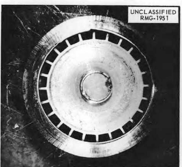
Fig. 4.1.7. Forward Face of Impeller from Pump Used in MTR In-Pile Loop No. 5. \frac{1}{2} X.
