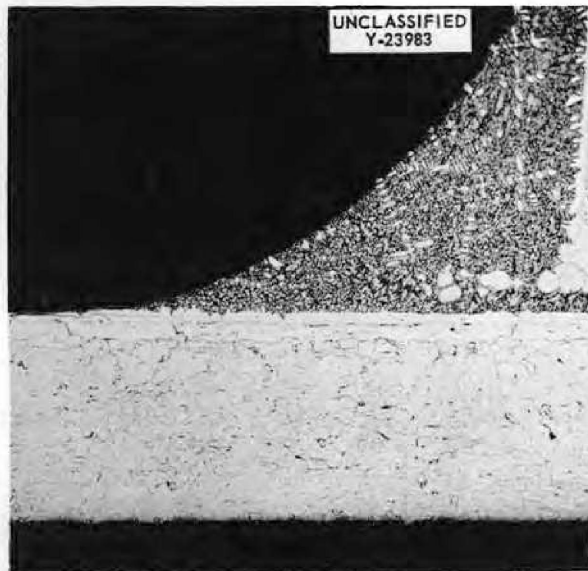
Fig. 3.3.18. Section Taken near Brazed Fillet To Show Small Grain Size of Carburized Tubing.
