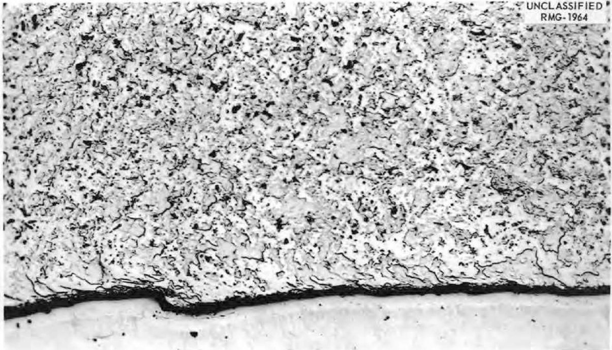
Fig. 4.1.14. Interior Surface of Molybdenum Jacket Removed from an Irradiated Zirconium Hydride-Containing Capsule. Specimen nickel-plated for edge preservation. 250X.
