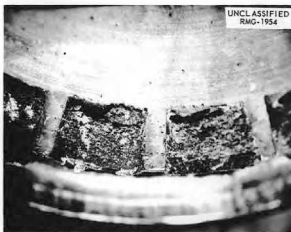
Fig. 4.1.10. Fuel Deposit Indicated by Arrow in Fig. 4.1.9 at a Higher Magnification. 4X .
