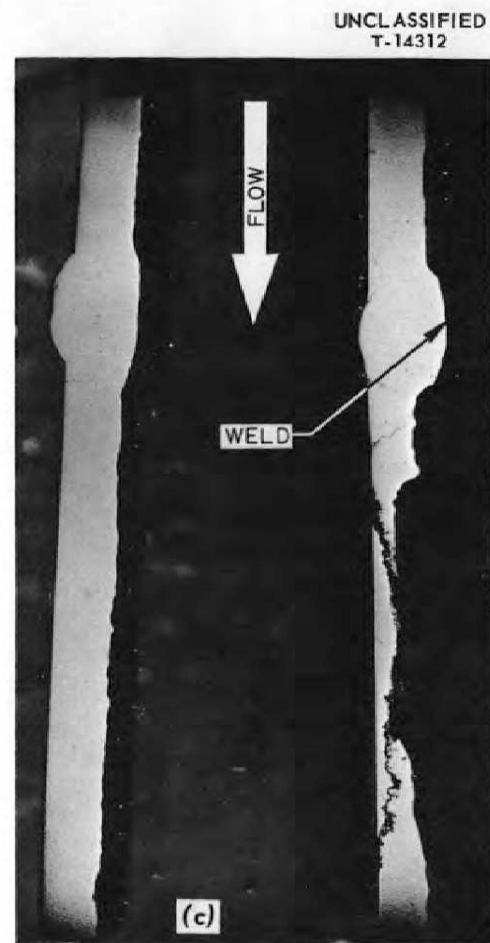
Fig. 1.7.2. Effect of High-Frequency Thermal Cycling on Inconel in an \text{NaF-ZrF}_4\text{-UF}_4 (56-39-5 Mole %) Environment – Test Run 5. (a) Inlet transition section; sample location e. 4X. (b) Section from sample location b; crack extends about 0.070 in. into 0.250-in. wall. 50X. (c) Exit region; sample location c; \frac{3}{8} -in. sched-40 pipe. 4X. (Secret with caption)
