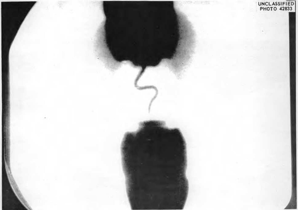
Fig. 3.7.1. Radiograph of a Semiconductor Diode ( \frac{3}{16} -in.-dia, \frac{5}{16} -in.-long) Made by Photographing the Monitor Screen of the X-Ray-Sensitive Television System.
