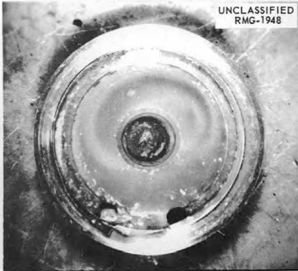
Fig. 4.1.4. Cover Plate of Housing for Impeller of Pump Used in MTR In-Pile Loop No. 4. \frac{1}{2} X.
